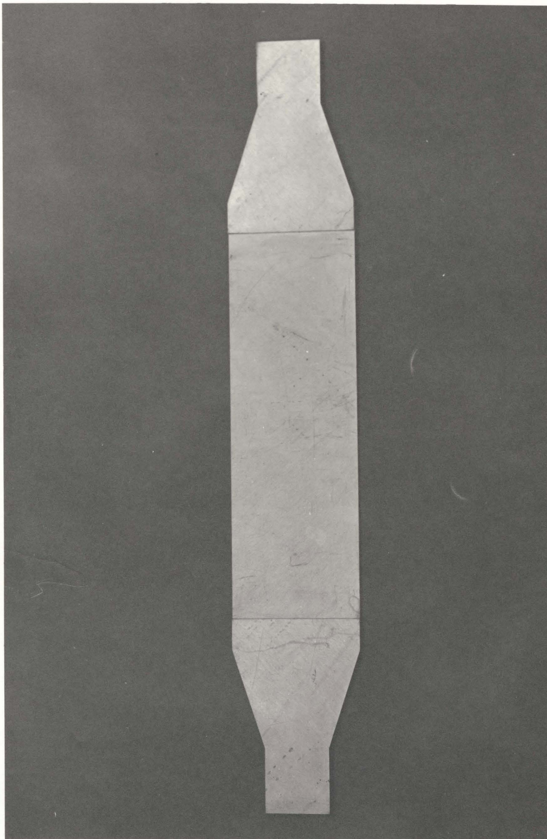
PHOTOGRAPH 3.1 MAIN SPECIMEN FOR SHEET-STRETCHING TEST
