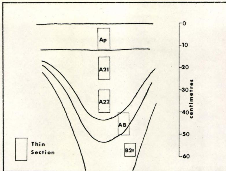
Fig. 3. Location of thin sections in soil tongue at Freelton.
