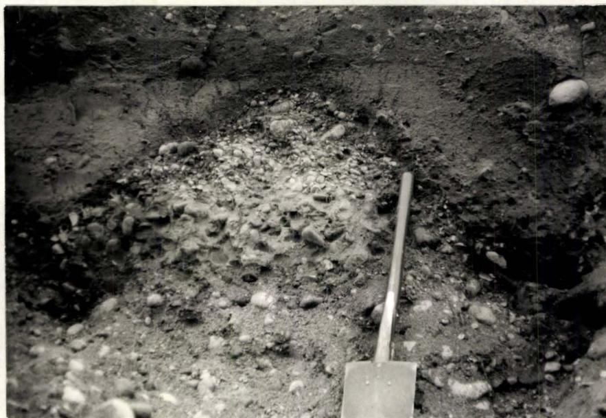
Fig. 46 Compacted and disturbed layer of gravel at Bridgeport.
