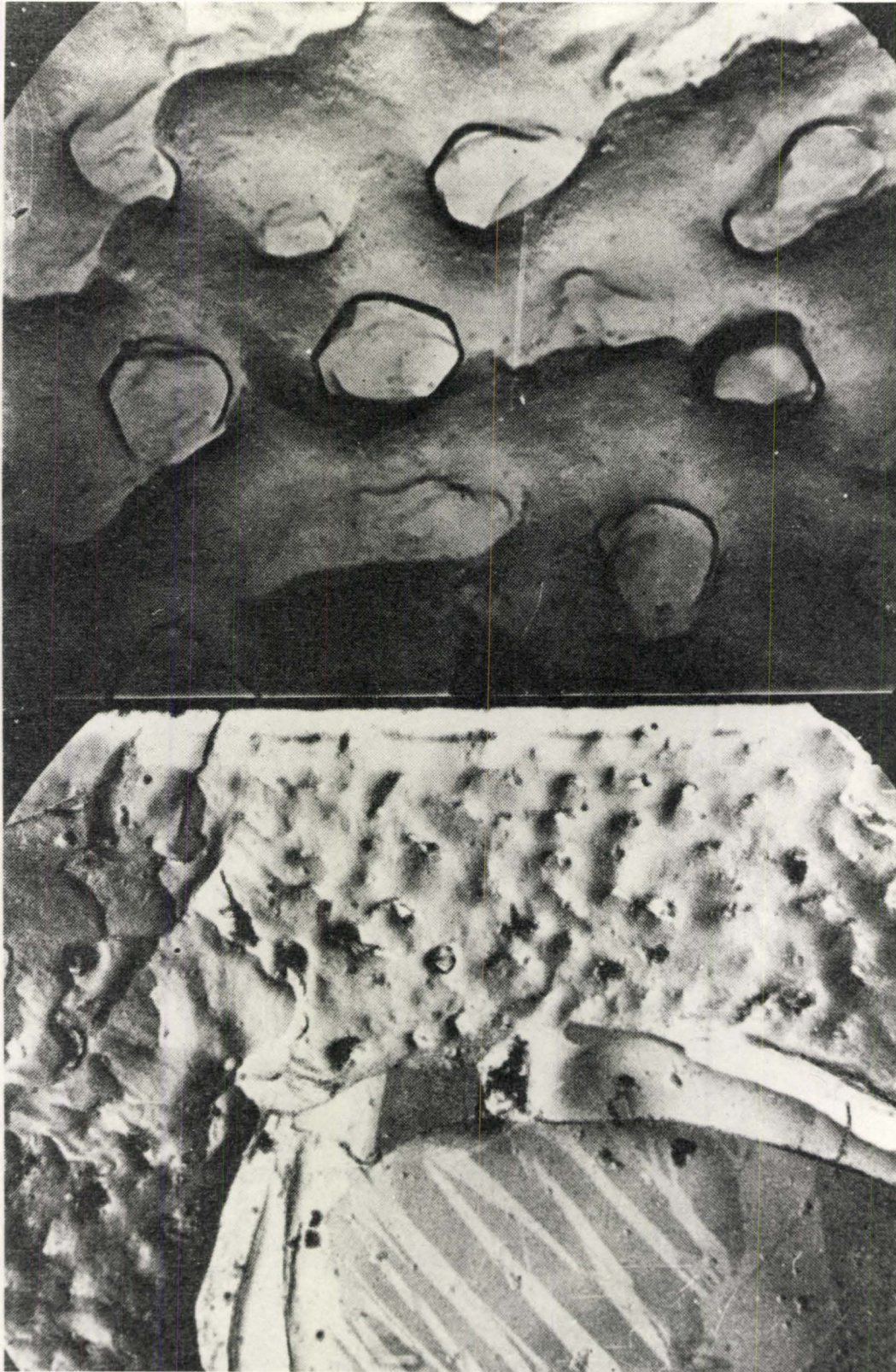
Figure 18. Electron Micrographs of As-Fired Replica Illustrating Multi-phase Microstructure. After Jaeger and Nickell [107].
