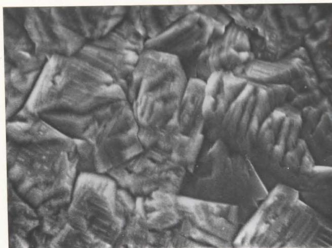
Exposure: 20 min. at 800°C in oxygen at 0.30 torr (X1650).
