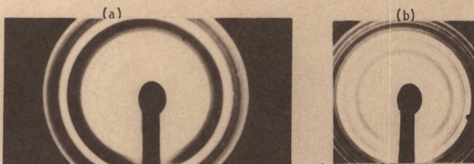
Figure 11. Diffraction Patterns ((a) 80KV, (b) 100KV) of specimens heated at 650°C (a) and 800°C (b).
