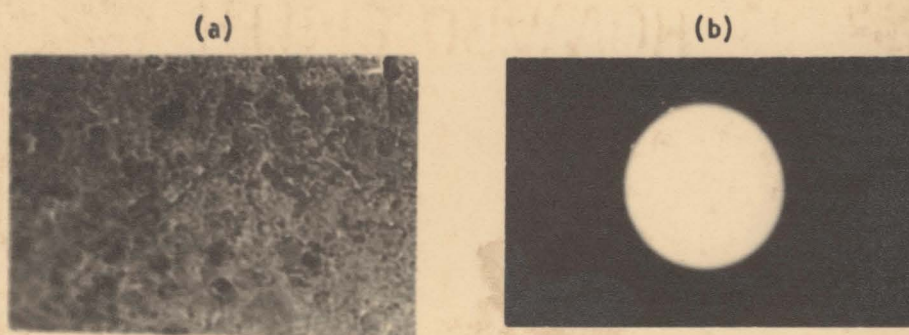
Figure 30. (a) Transmission and (b) diffraction micrographs of \text{SnO}_2 films after bombardment with 35 keV krypton ions. Dose = 10 \mu\text{A} \times 30 \text{ sec/cm}^2 . magn. 2.5 \times 10^4 -100KV.
