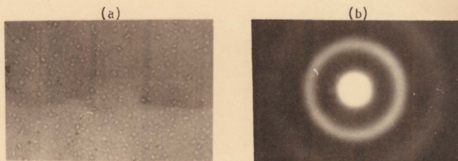
Figure 38. (a) Transmission and (b) diffraction micrographs of \text{SnO}_2 film after bombardment with 35 keV krypton ions for 30 min. Current \leq 10 \mu\text{A} magn. 10^4 -80KV.
