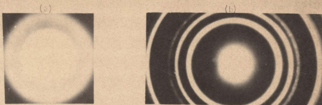
Figure 5. Diffraction Patterns ((a) 80 KV, (b) 60 KV) of films obtained by ion-beam sputtering of \text{SnO}_2 , with cooled target. (a) as deposited (b) after pulse heating.
