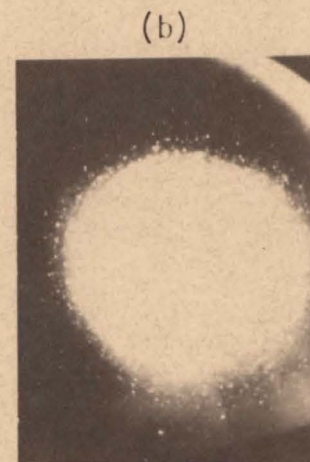
Figure 17. (a) Transmission electron micrograph and (b) electron diffraction pattern of \text{SnO}_2 film deposited on water cooled substrates.
