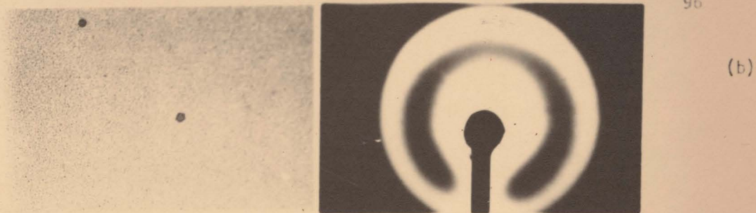
Figure 43. (a) Transmission and (b) diffraction micrographs of reactively sputtered \text{SnO}_2 film. Sputtering time: 15 min. (4mA-2KV). magn. 11,000-80KV. (60mA/min).
