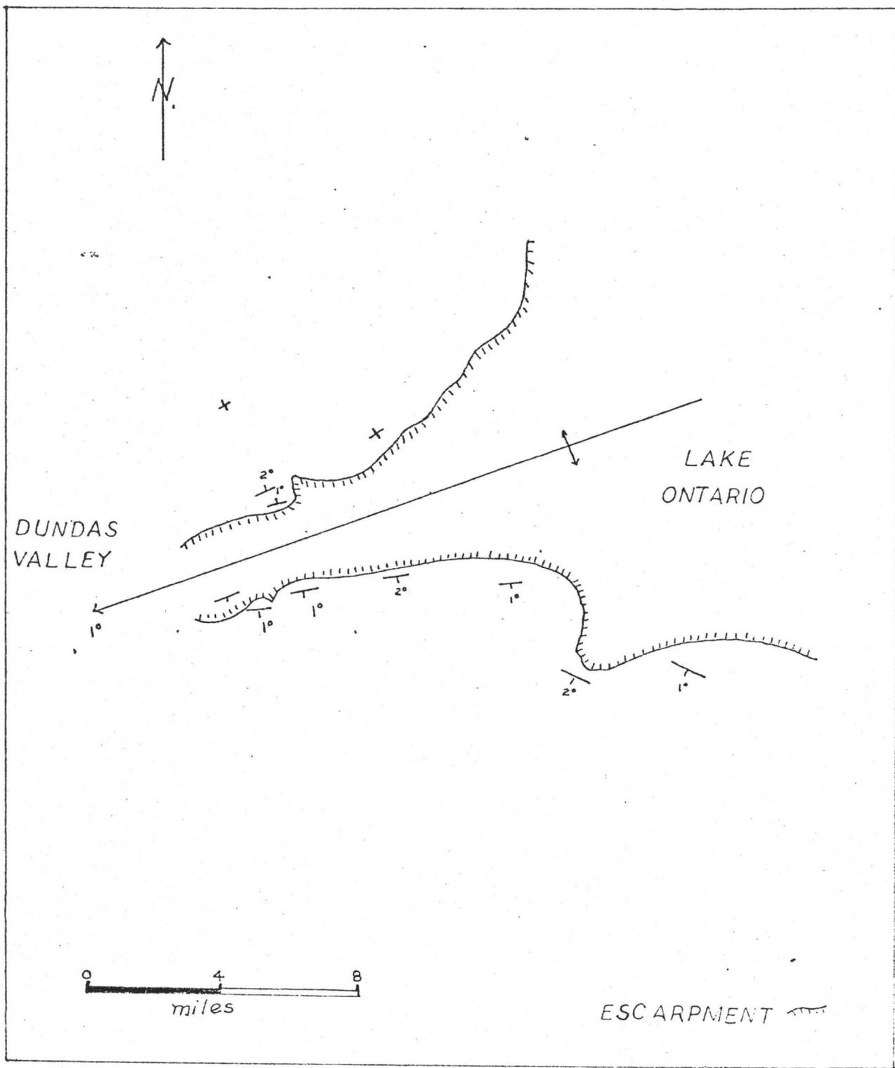
Fig. 2.2a Map of core altitudes and proposed anticlinal axis (after Hurst).
