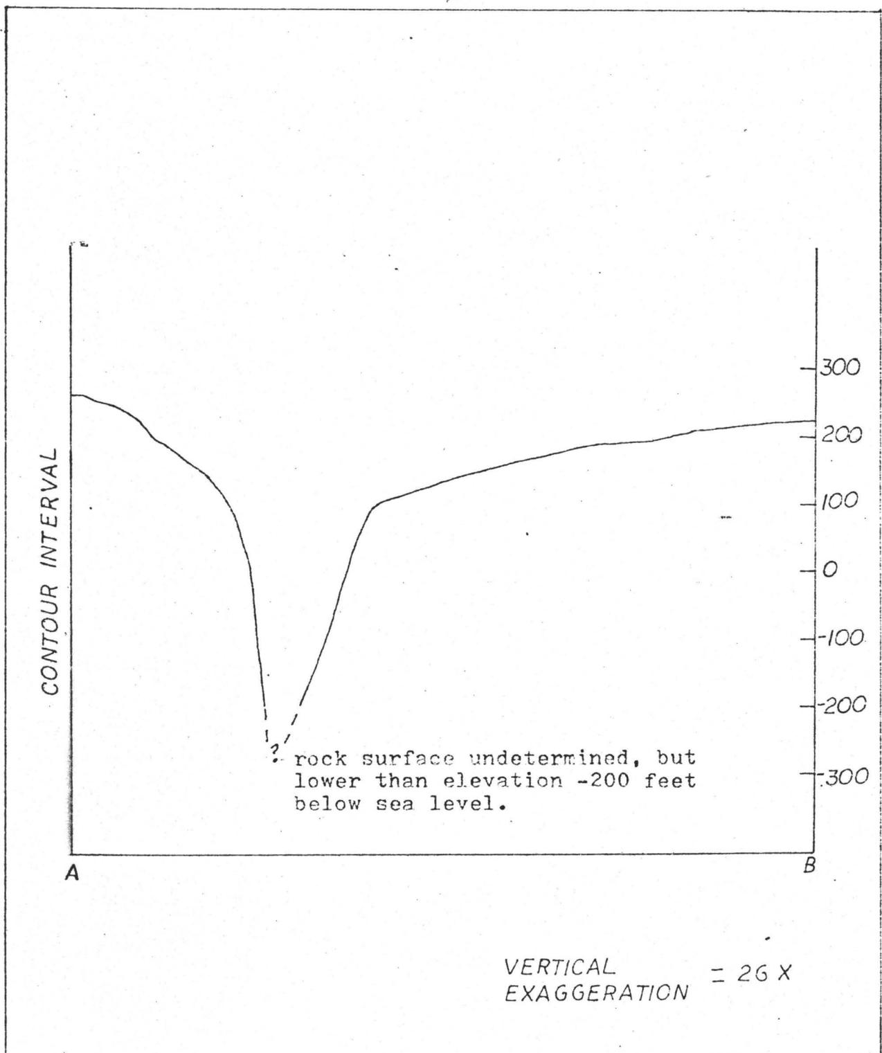
Fig 2:2 Bedrock Contour Cross Section Across The Burlington Bar
