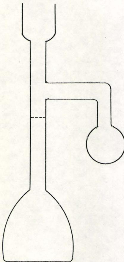
Figure 8. Reaction flask used for kinetics.
