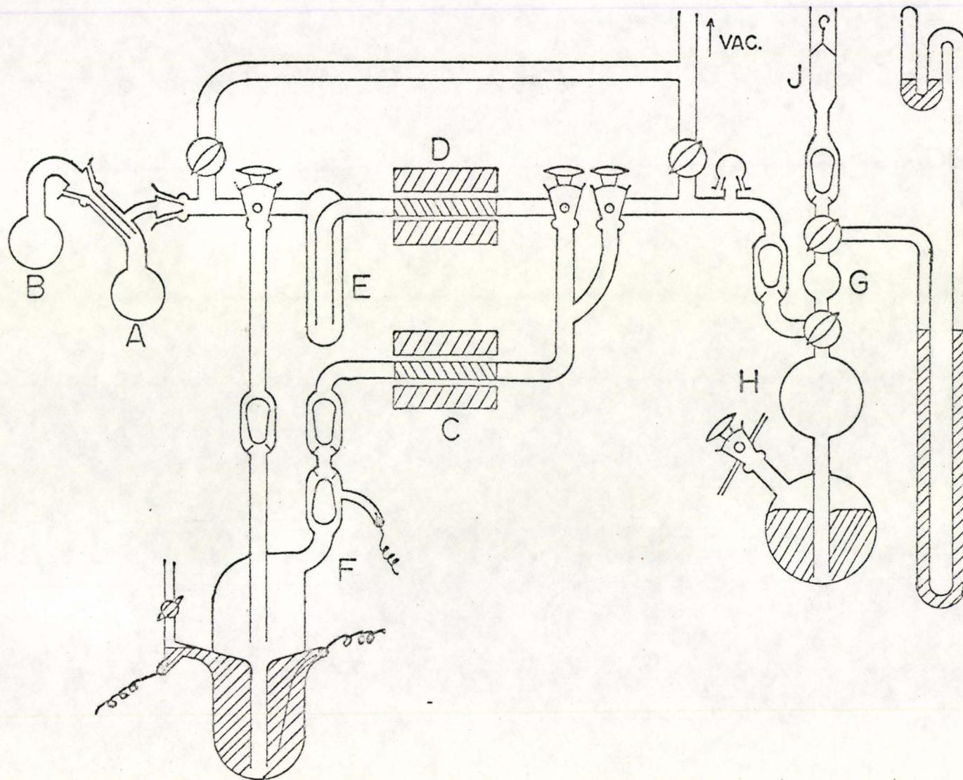
Fig. 10 APPARATUS USED FOR THE PREPARATION AND PURIFICATION OF NITROGEN SAMPLES.
