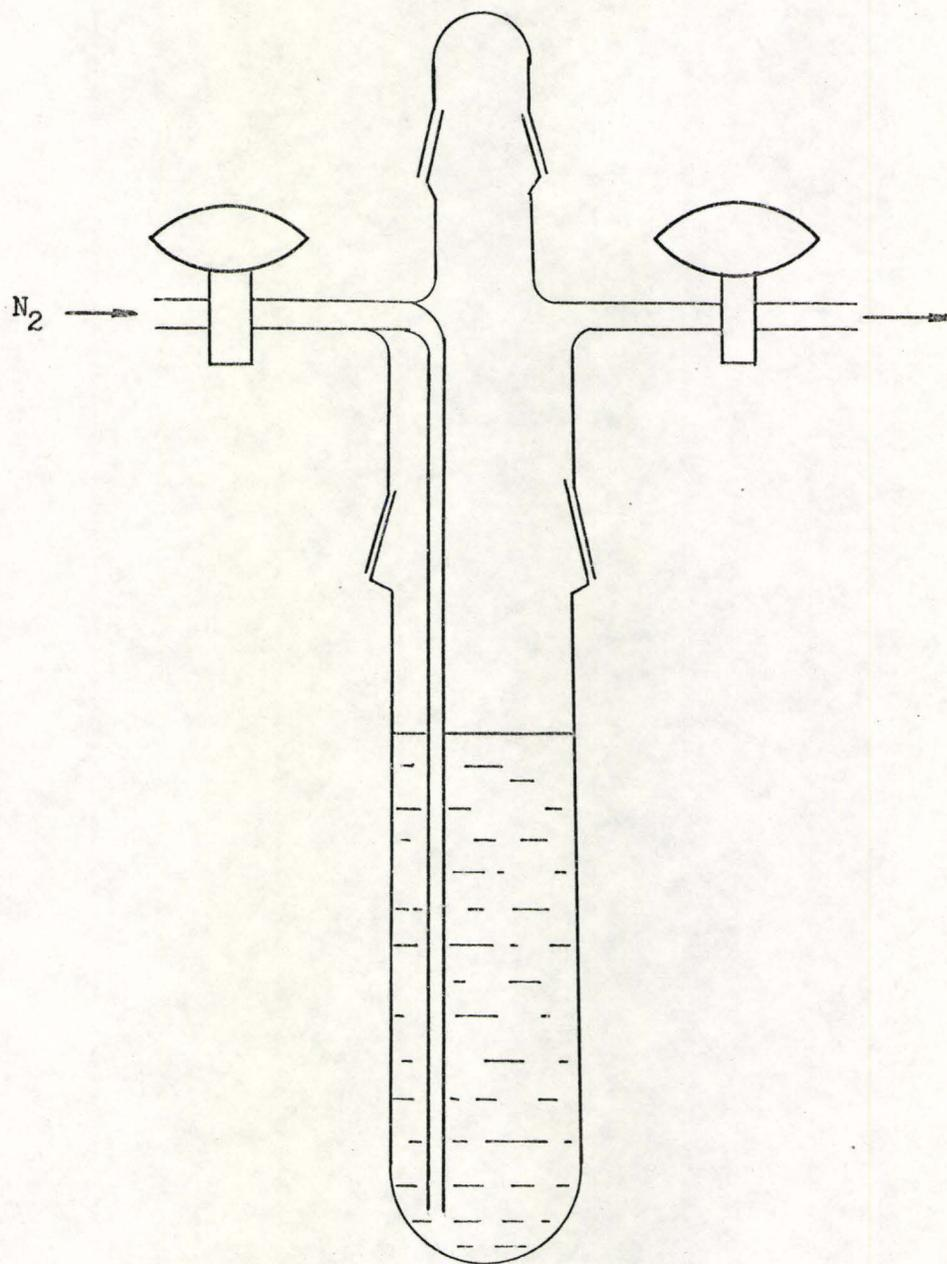
Figure. 7 Apparatus for the preparation and storage of stock sodium ethoxide solutions.
