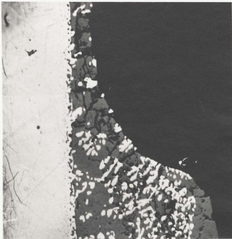
Figure 28. Typical ring of iron formed at the melt surface due to heat abstraction.
