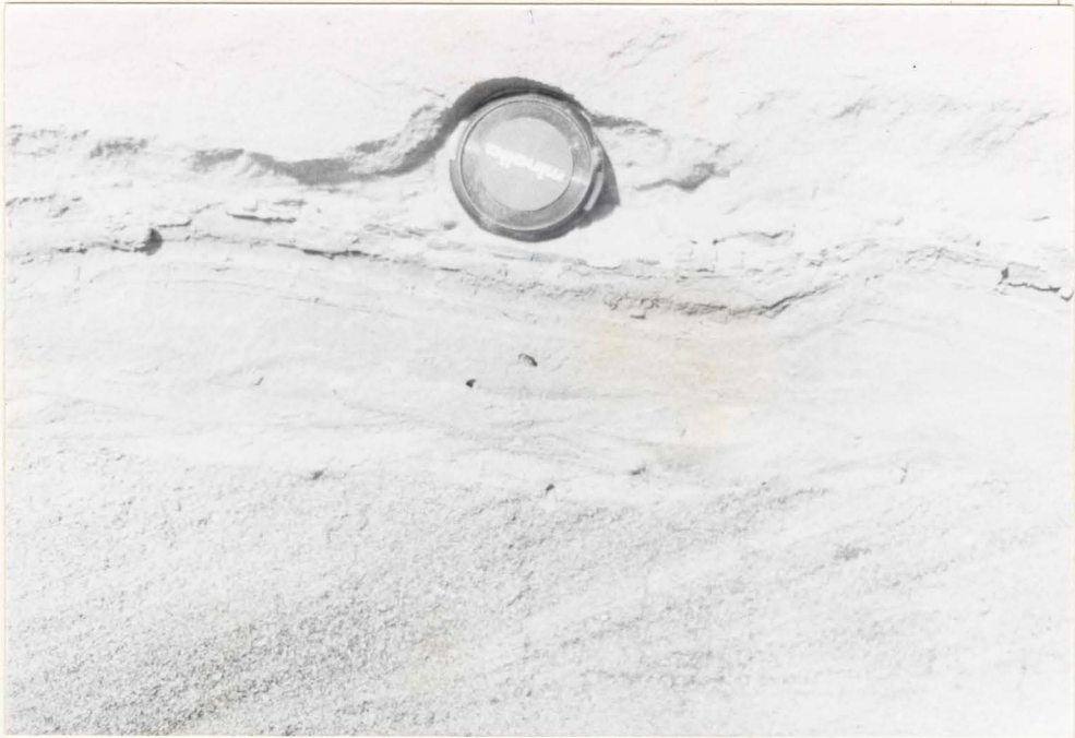
Figure 3.6 Sequence of facies moving from cross-bedded sand to trough-shaped small-scale cross-lamination to draped lamination. Flow strength decreases upwards.
