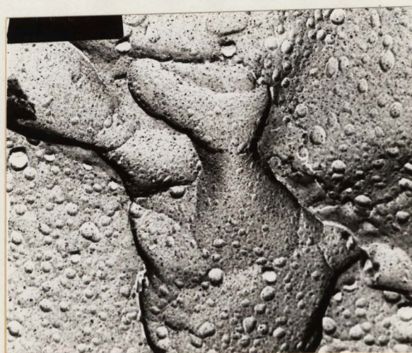
Figure 24. Replicas of PSZ sample thermally shocked from 1200°C into a blast of cold air for (a) one cycle, (b) 5 cycles, (c) 10 cycles.
