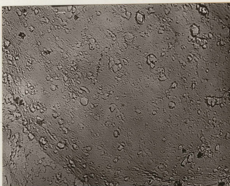
(b) Replica of PSZ thermally shocked from 800°C into a blast of cold air for one cycle (batch #1).
