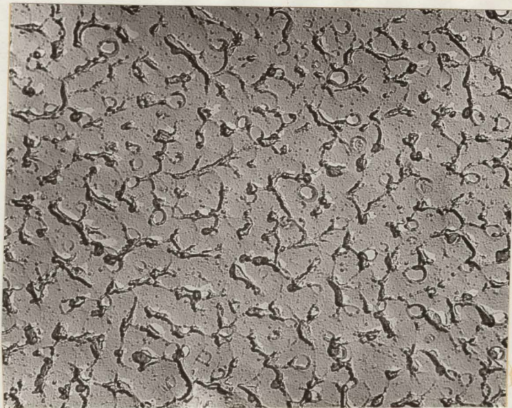
(b) Replica of PSZ sample shocked from 1200°C into a blast of cold air for one cycle.
