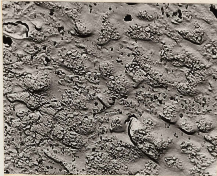
(a) Replica of PSZ sample shocked from 1100°C into a blast of cold air for one cycle.
