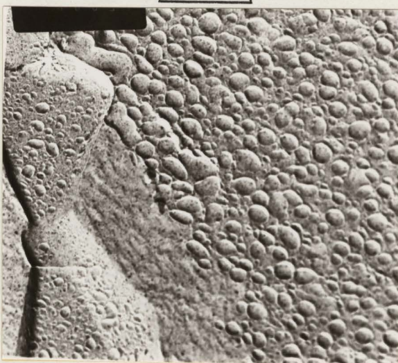
Figure 23. Replicas of PSZ sample thermally shocked from 1100^{\circ}\text{C} into a blast of cold air for (a) one cycle, (b) 5 cycles, (c) 10 cycles.
