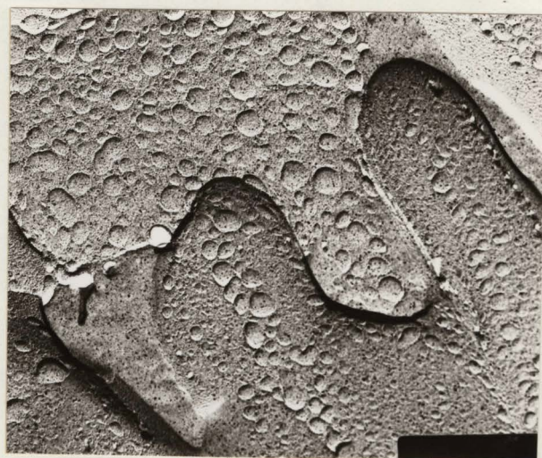
Figure 25. Replicas from PSZ sample thermally shocked from 1300°C into a blast of cold air for (a) one cycle, (b) 3 cycles, and (c) 7 cycles.
