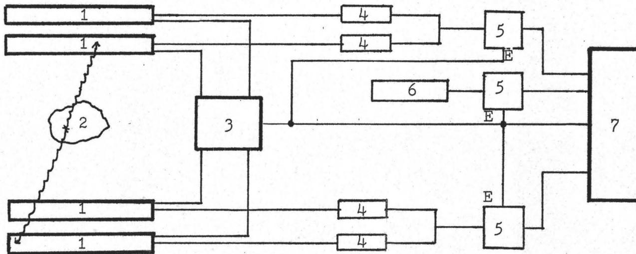
Figure 1. Basic Details of Positron Camera
