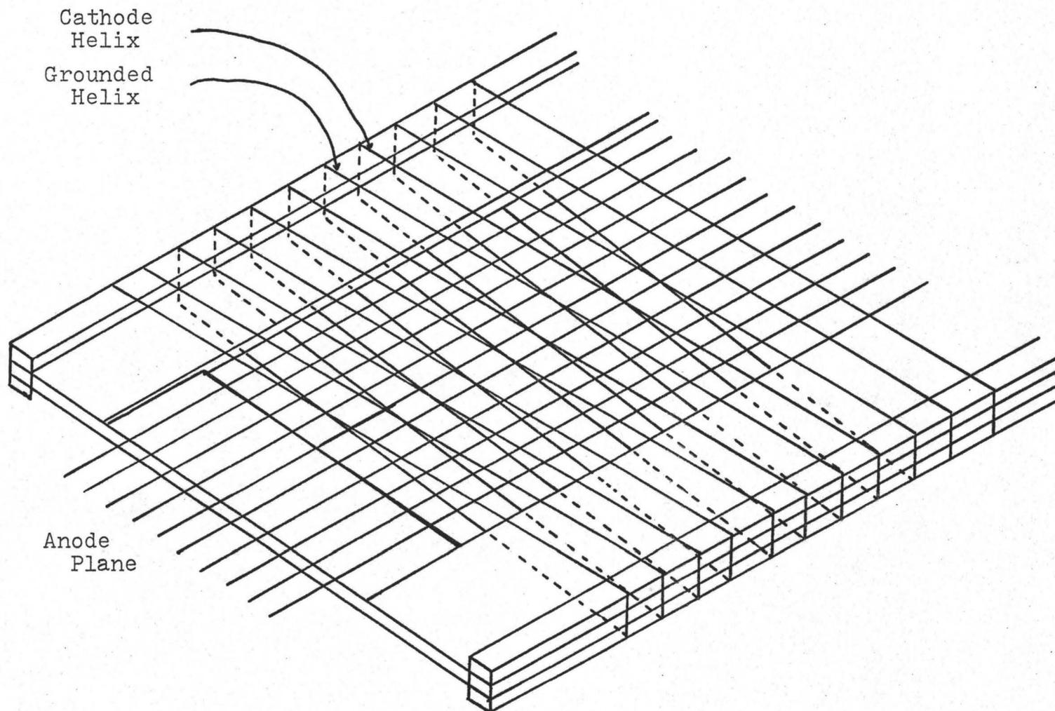
Figure 2. Bifilar Helical Cathode MWPC Windings
