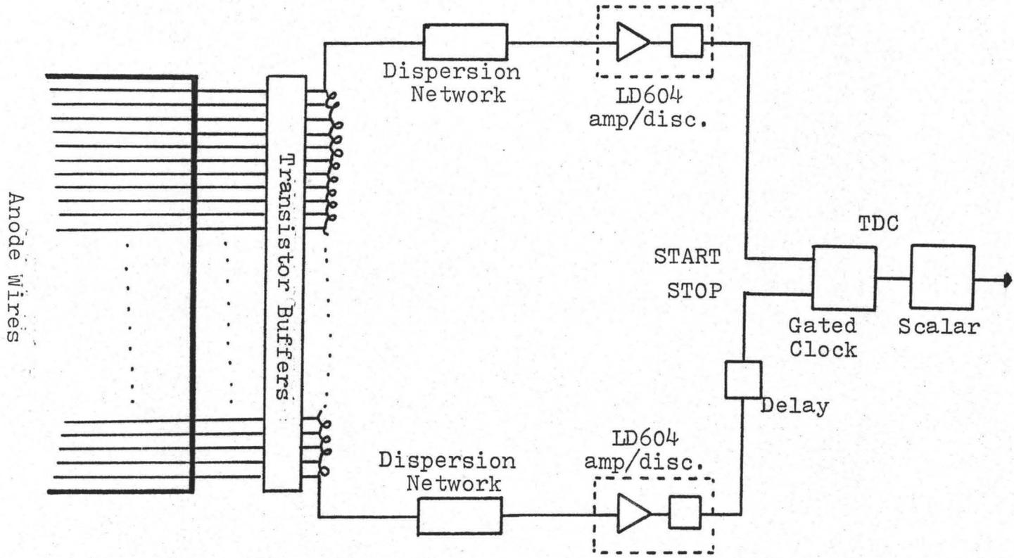
Figure 3. Anode Readout System
