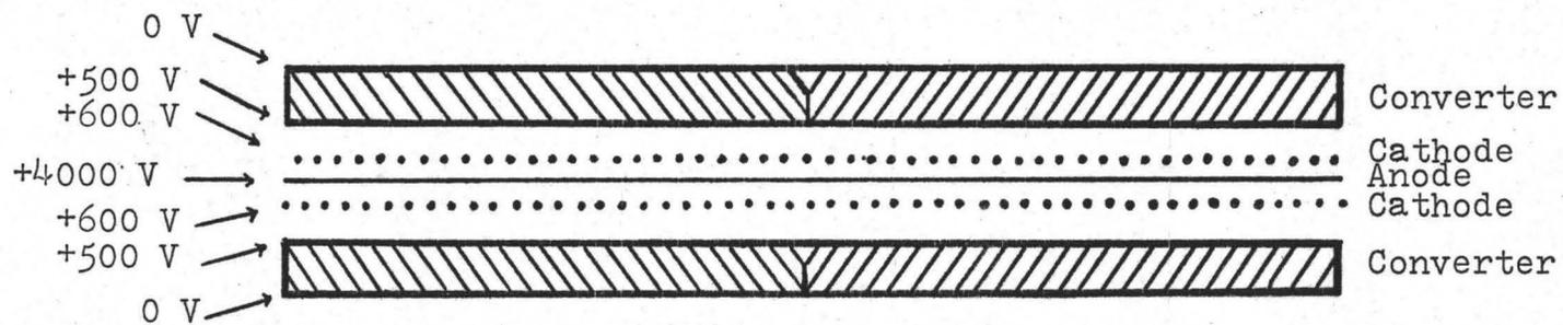
Figure 6. MWPC Fitted With Converter Plates
