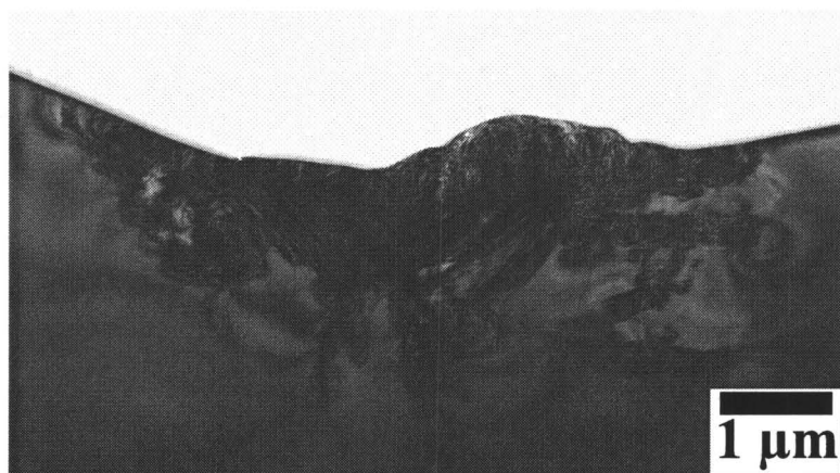
Figure 7.10: Cross-sectional bright-field TEM image of the specimen irradiated by a single high-fluence ( 33 \text{ J/cm}^2 ) pulse, shown in figure 7.1(d). This image is from reference [45].
