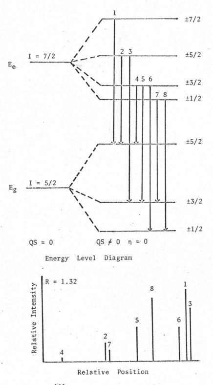
Figure 1. <sup>121</sup>Sb Quadrupole Interaction.
