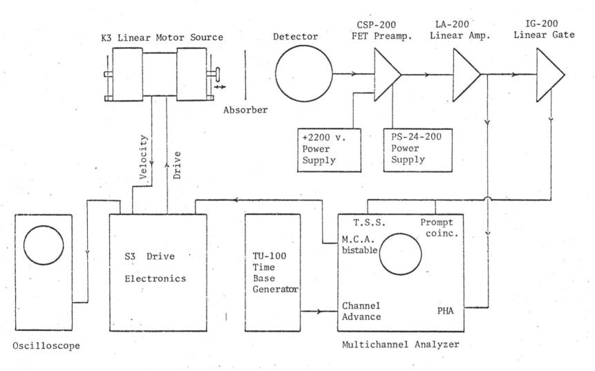
Figure 2. Mössbauer Spectrometer - Block Diagram
