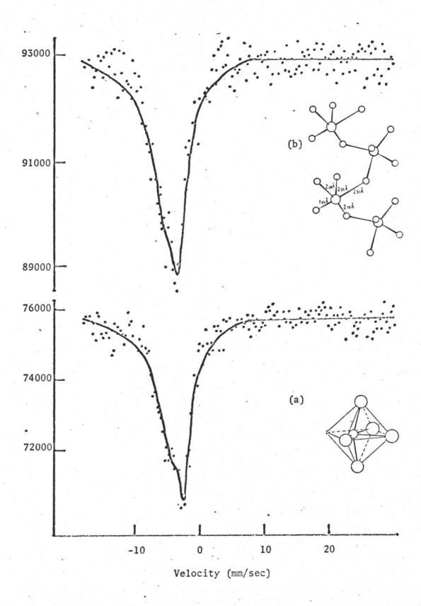
Figure 7. Mössbauer Spectra: (a)  $K_2SbF_5$ , (b) NaSbF<sub>4</sub>.
