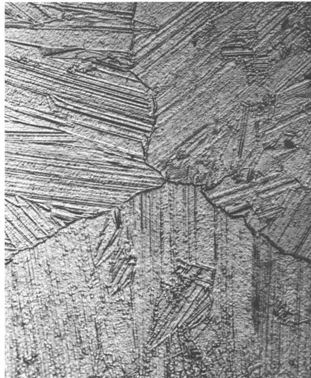
Figure 6.14. Micrograph of polycrystalline Si X625, CP-4 etch. (perpendicular to growth direction)
