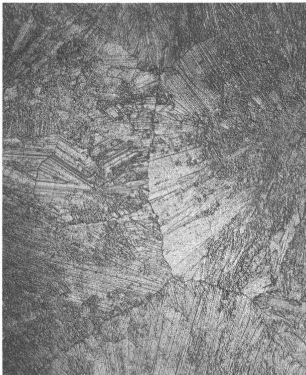
Figure 6.13. Micrograph of polycrystalline Si X200, CP-4 etch. (perpendicular to growth direction)
