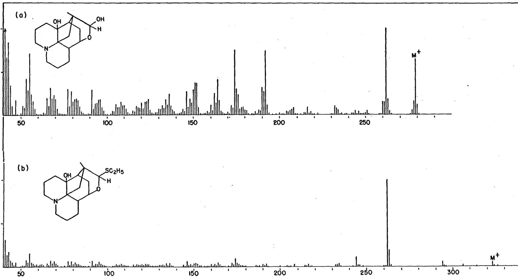
Figure 9. The Mass Spectrum of (a) Dihydrocannotinol (b) Compound X
