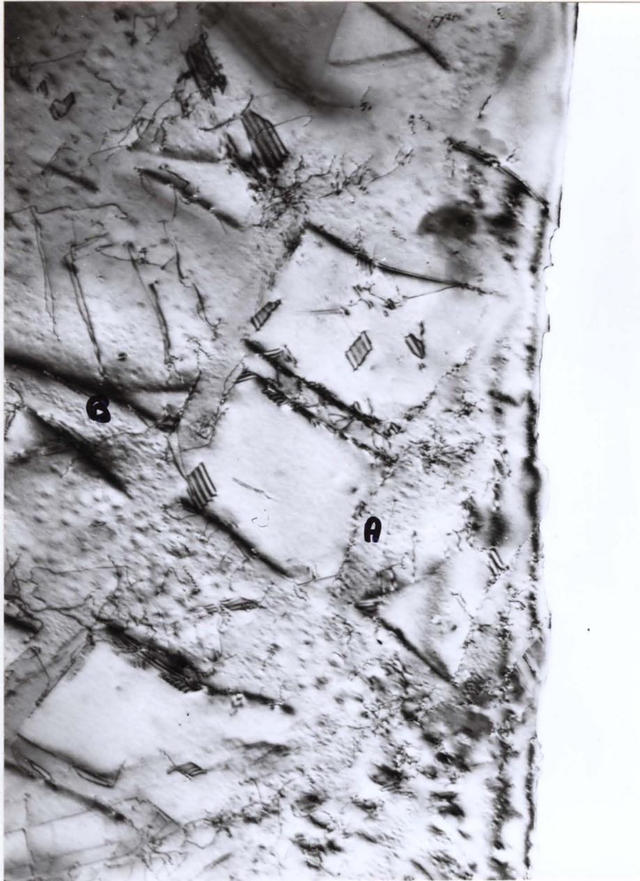
Fig. 38: Transmission electron micrograph of (100) section from 17<sup>a</sup>/o Al single crystal, slow cooled 1300 to 700°C in 3 hours and compressed 5%.
