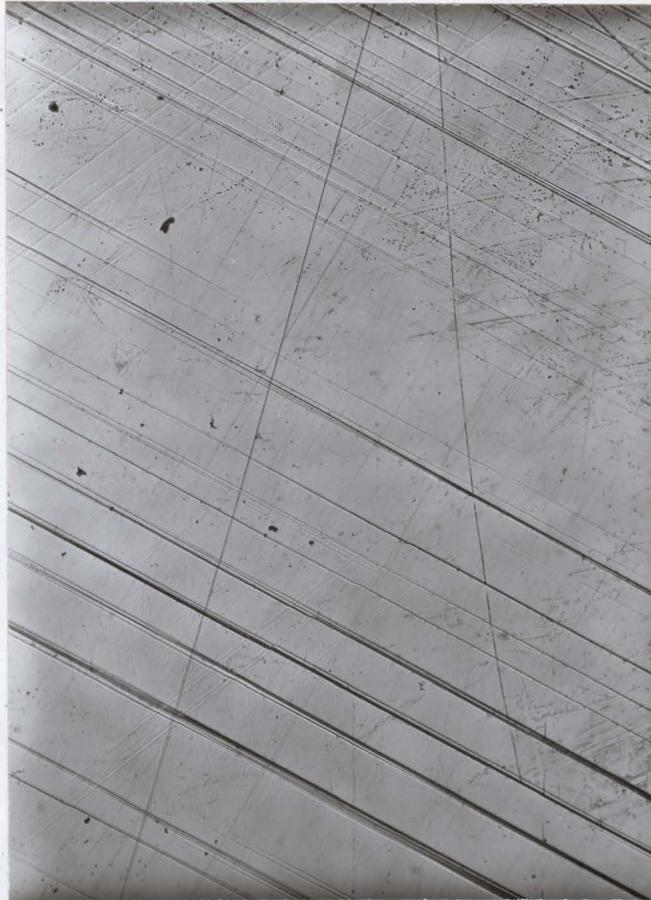
Fig. 26: Surface slip line structure of 17<sup>a</sup>/o Al single crystal aged 700<sup>o</sup>C for 6 hours and compressed 4%.
