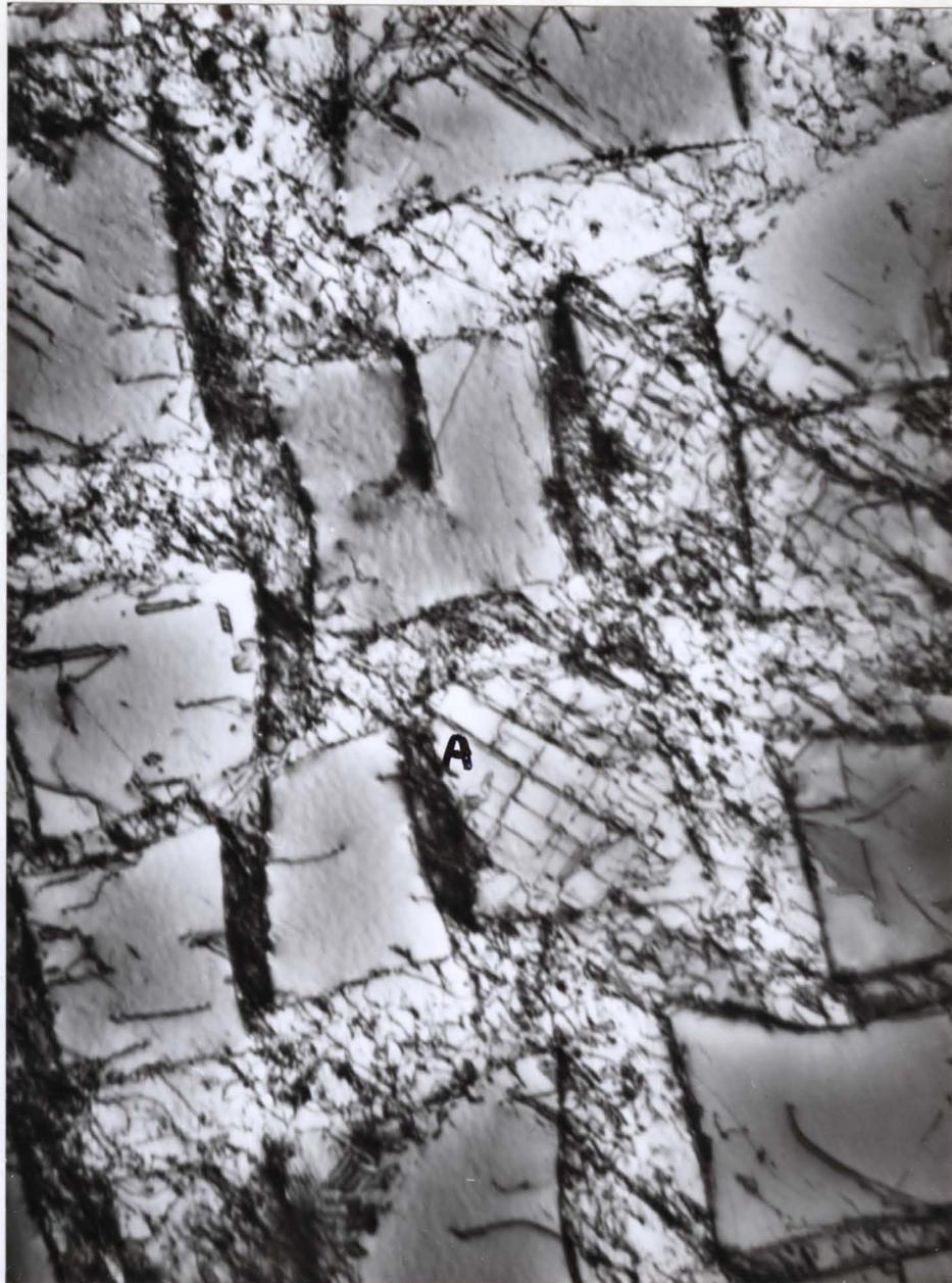
Fig. 39: Transmission electron micrograph of (100) section of 17<sup>a</sup>/o Al single crystal, slow cooled 1300 to 700°C in 3 hours, cold rolled 3%. X35,000
