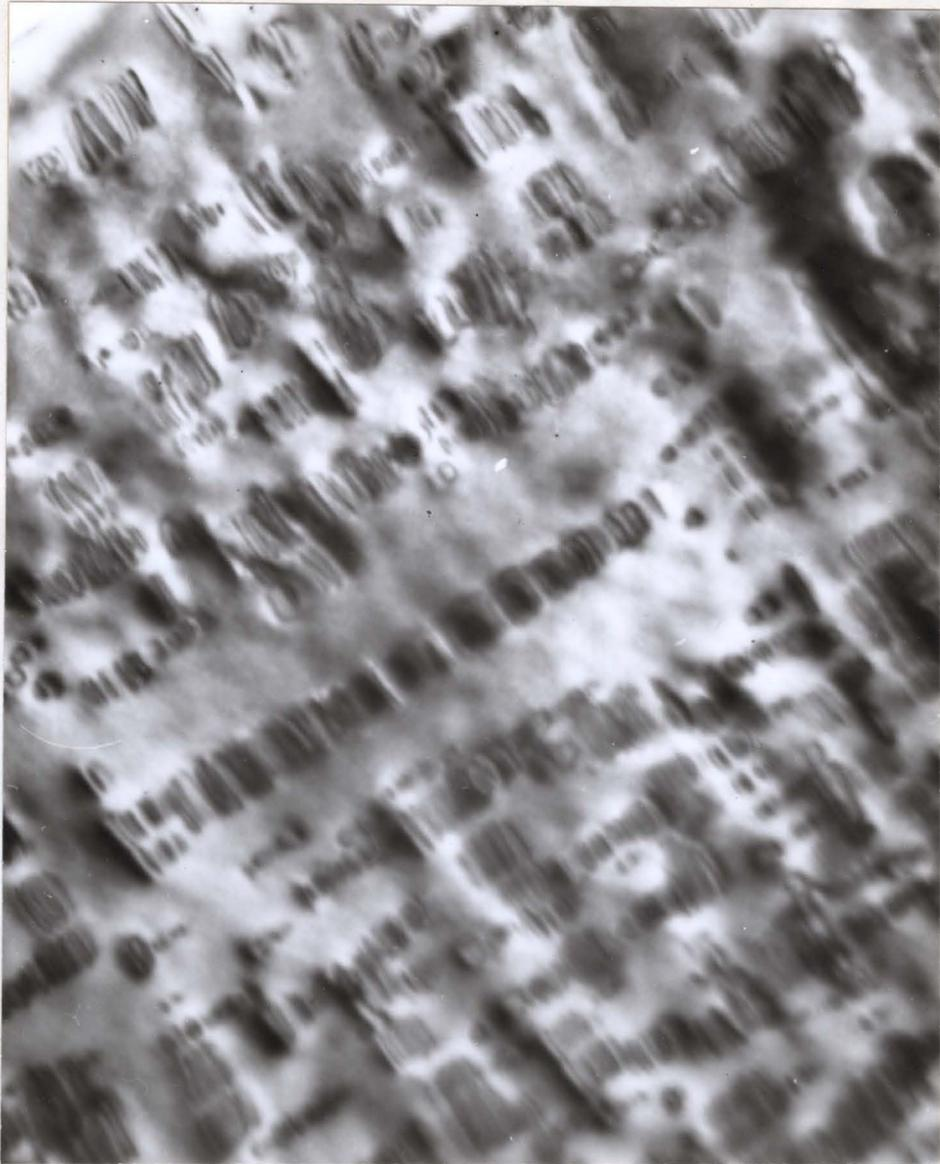
Fig. 56: Transmission electron micrograph of 13<sup>a</sup>/o Al single crystal
