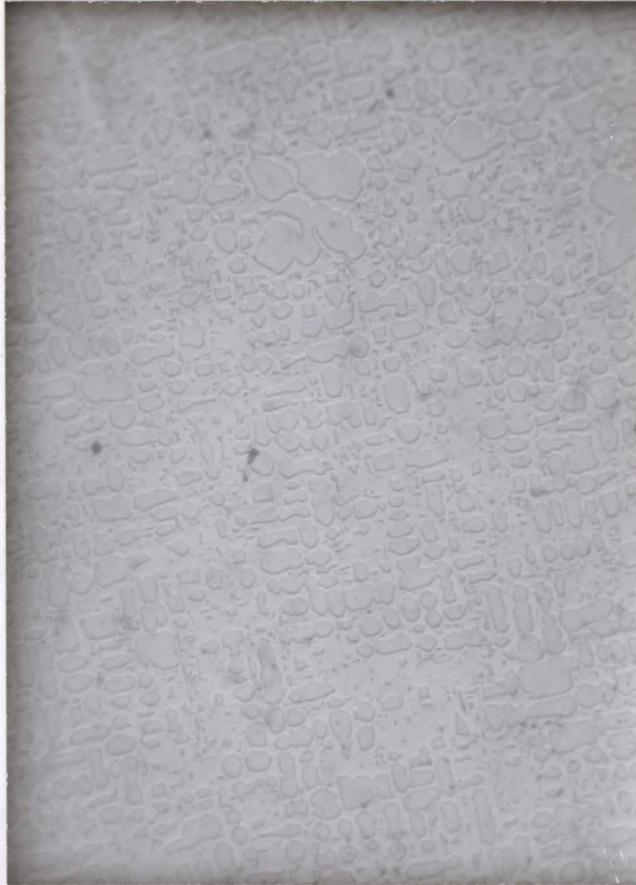
Fig. 47: Optical micrograph of (100) section from 17<sup>a</sup>/o Al single crystal, step cooled 1300 to 700<sup>o</sup>C over 3 weeks. X750
