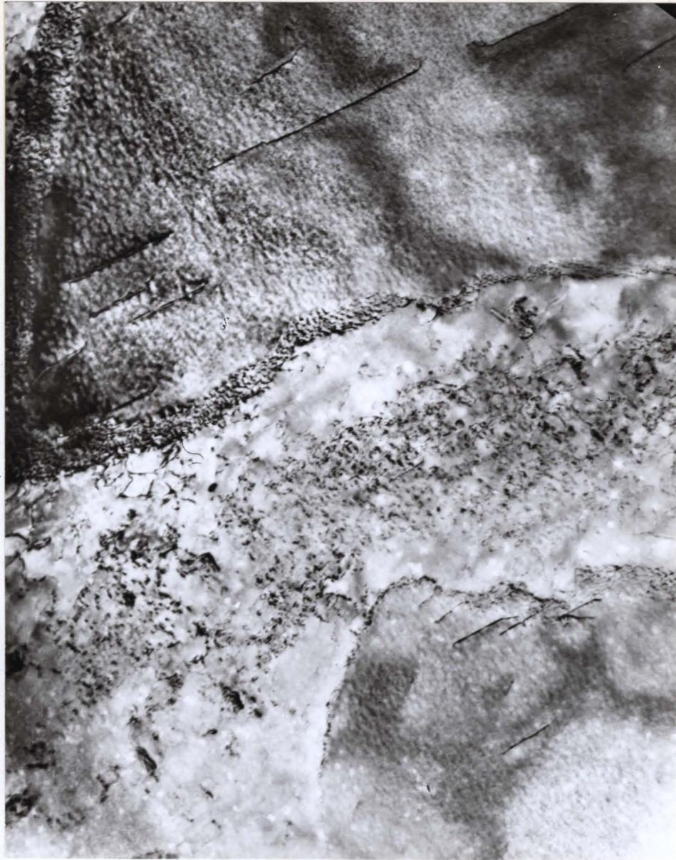
Fig. 54: Transmission electron micrograph of 18<sup>a</sup>/o Al single crystal slow cooled 1300 to 700<sup>o</sup>C in 3 hours. X32,000
