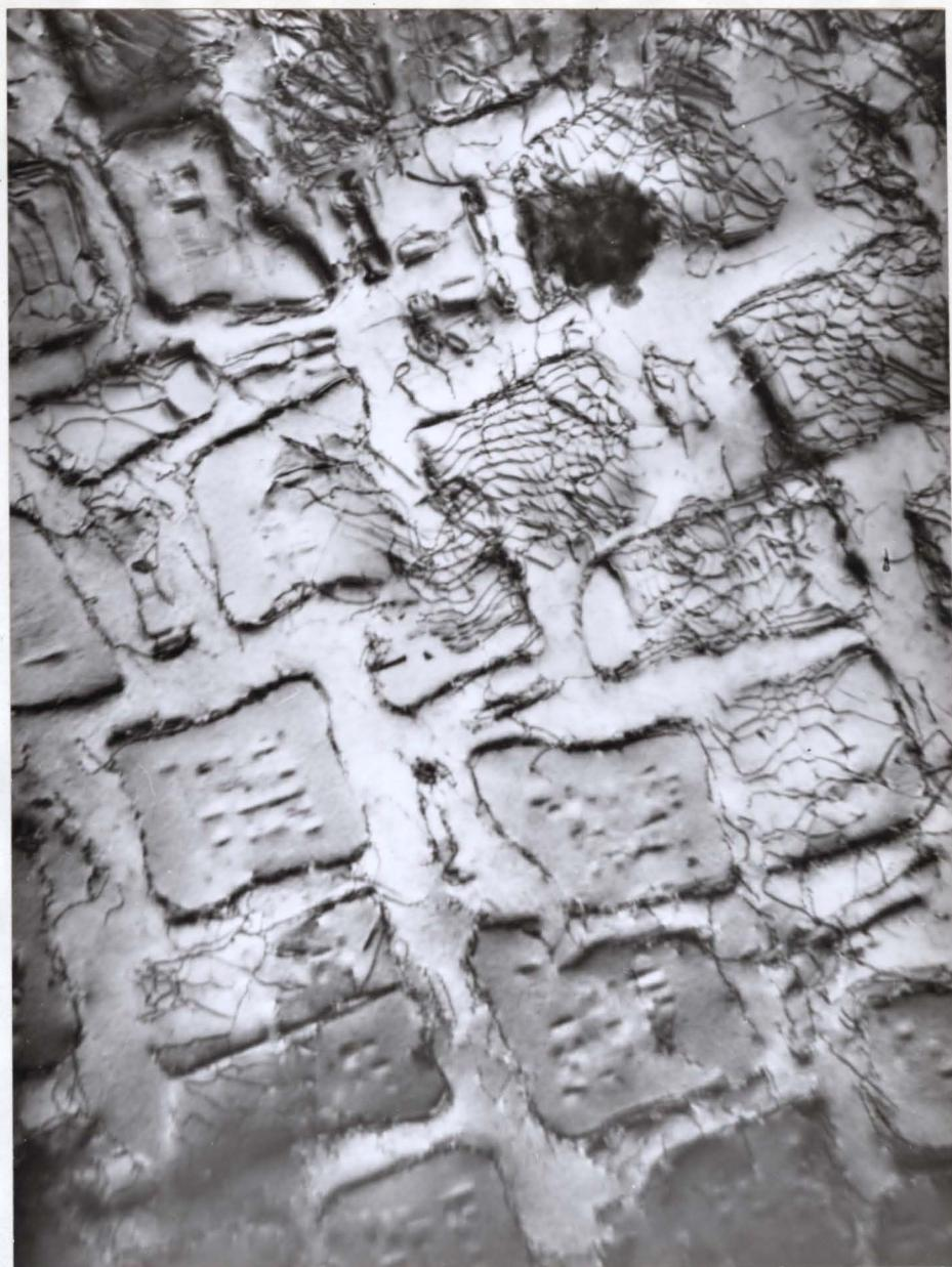
Fig. 46: Transmission electron micrograph of (100) section from 17<sup>a</sup>/o Al single crystal slow cooled 1300 to 700<sup>o</sup>C in 3 hours and aged 4 weeks at 700<sup>o</sup>C. X20,000
