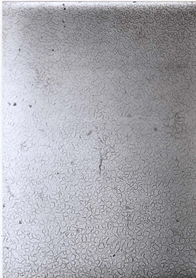
Fig. 53: Optical micrograph of surface of 18<sup>a</sup>/o Al single crystal
