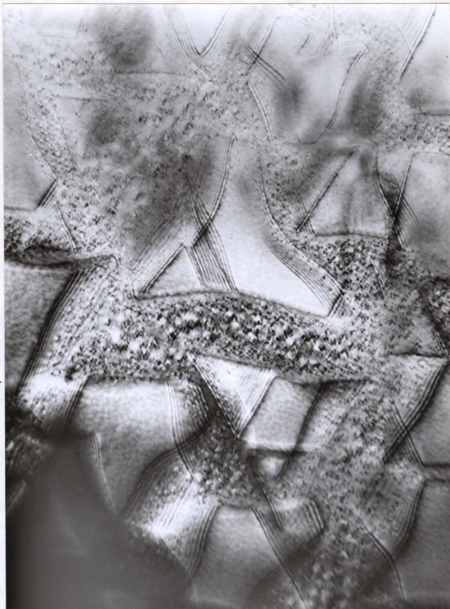
Fig. 37: Transmission electron micrograph of (111) section from 17<sup>a</sup>/o Al single crystal slow cooled 1300-700<sup>o</sup>C in 3 hours and compressed 2% strain. Showing overlapping  $\delta$ -fringes. X24,000
