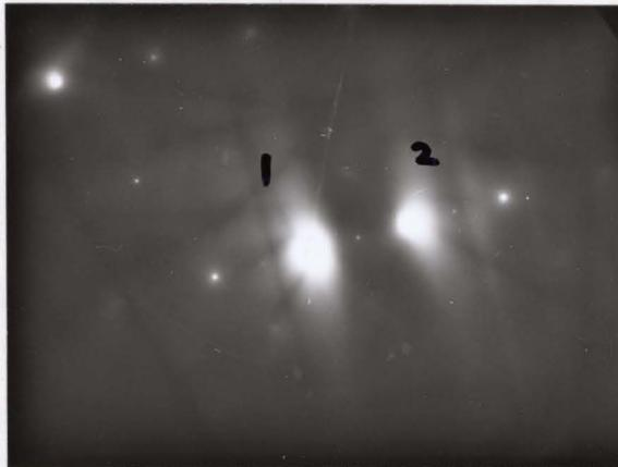
Fig. 21: Electron diffraction patterns showing shift in Kikuchi lines denoting change in orientation on crossing clear zones (see Fig. 20).
