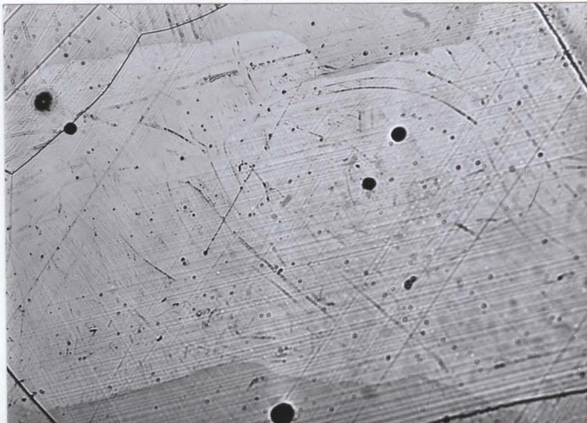
Fig. 61: Optical micrograph of pure Ni<sub>3</sub>Al polycrystalline alloy compressed 1%. X288
