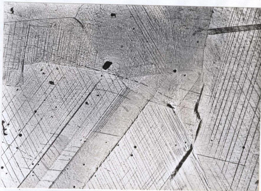
Fig. 64: Optical micrograph of 14<sup>a</sup>% Al polycrystalline alloy aged 700<sup>o</sup>C ¼ hour, compressed 1%. Deformation in grain boundary regions. X160
