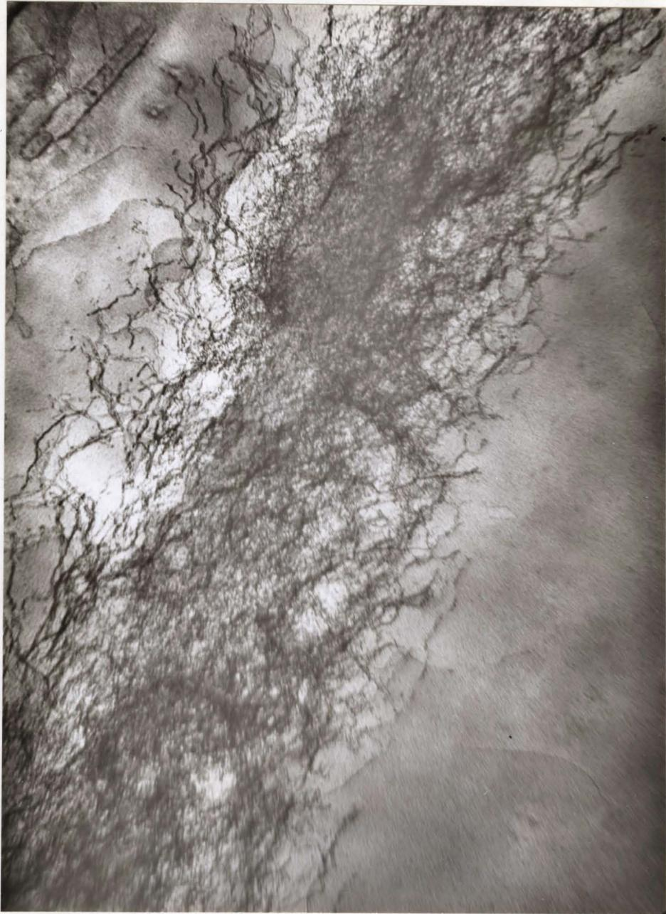
Fig. 22: Transmission electron micrograph from (111) section of 15<sup>a</sup>/o Al single crystal aged 700<sup>o</sup>C for 6 hours showing dislocation pairs in pile-ups associated with kink bands. X8,000
