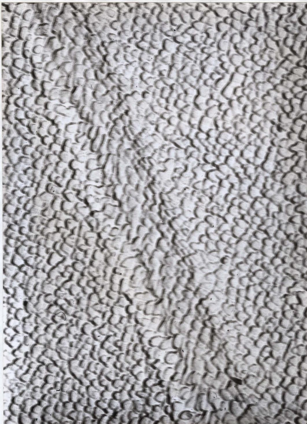
Fig. 33: Carbon replica of surface of 17<sup>a</sup>% Al single crystal, aged 700<sup>o</sup>C 6 hours, after 12% compressive strain. X60,000
