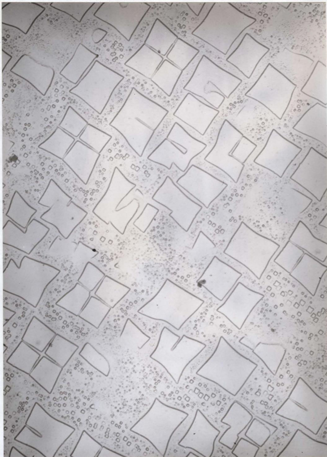
Fig. 34: Carbon replica of (100) section from 17<sup>a</sup>/o Al single crystal
