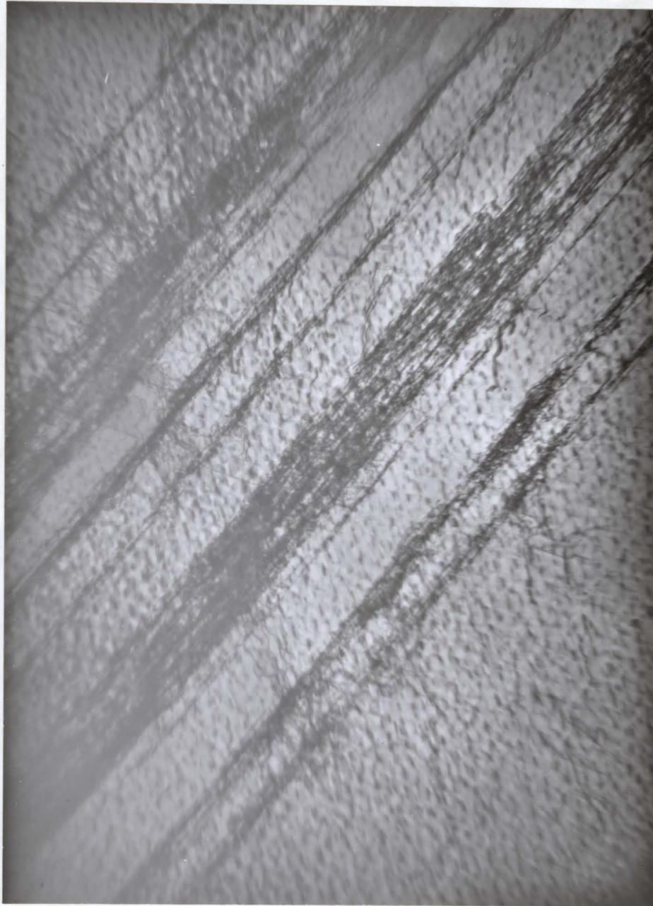
Fig. 32: Transmission electron micrograph of section perpendicular to (111) slip planes of 17<sup>a</sup>/o Al single crystal aged 700<sup>o</sup>C for 6 hours after 28% compressive strain. X10,000
