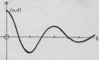
In the undamped case the period was  $\frac{2\pi}{A}$  and so the period is seen to be increased by damping.
