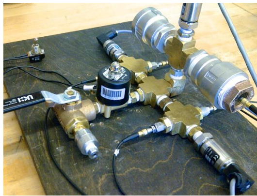
Figure B-2. Plenum chamber for pressure sensor calibration and response characterisation.
