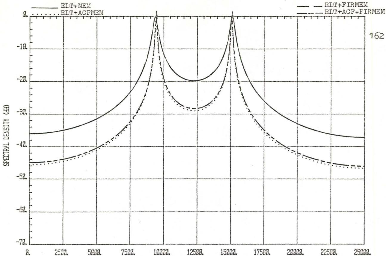
Fig. 4.31: The MEM spectra (filter order 4) of two sinusoidal-modulated signals with carrier frequencies 9448 Hz and 15039 Hz.
