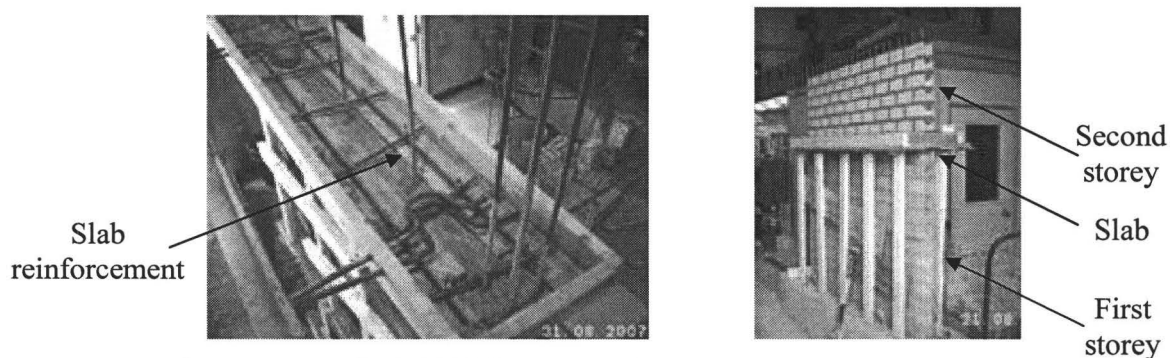
Fig. 2.7: Slabs representing the storey floors
