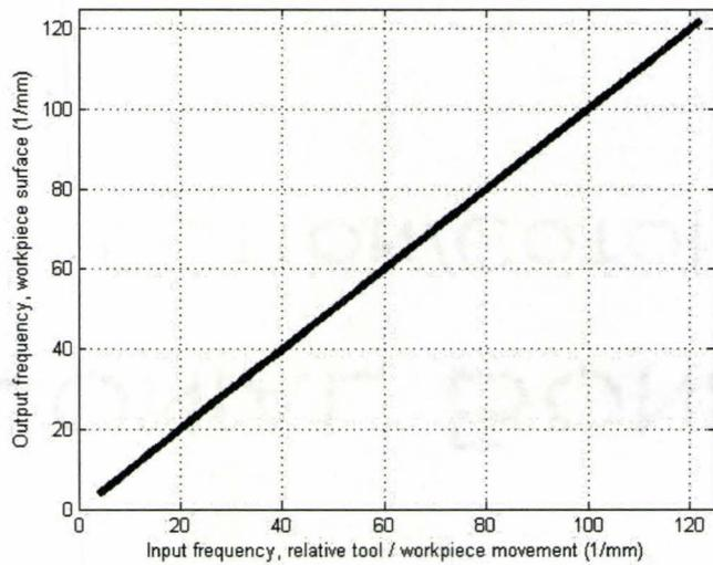
(a) Relative tool / workpiece spatial frequency and resulting spatial frequency on the cut workpiece surface, based on maximum FFT magnitude
