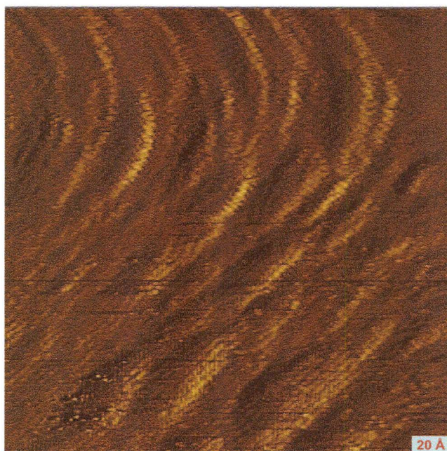
Figure 3.14: A 23.7 nm x 23.7 nm image of the annealed Au/mica spin-coated with Bingel SWCNTs taken with U_{SB} = -250 mV showing numerous bundles on the surface.
