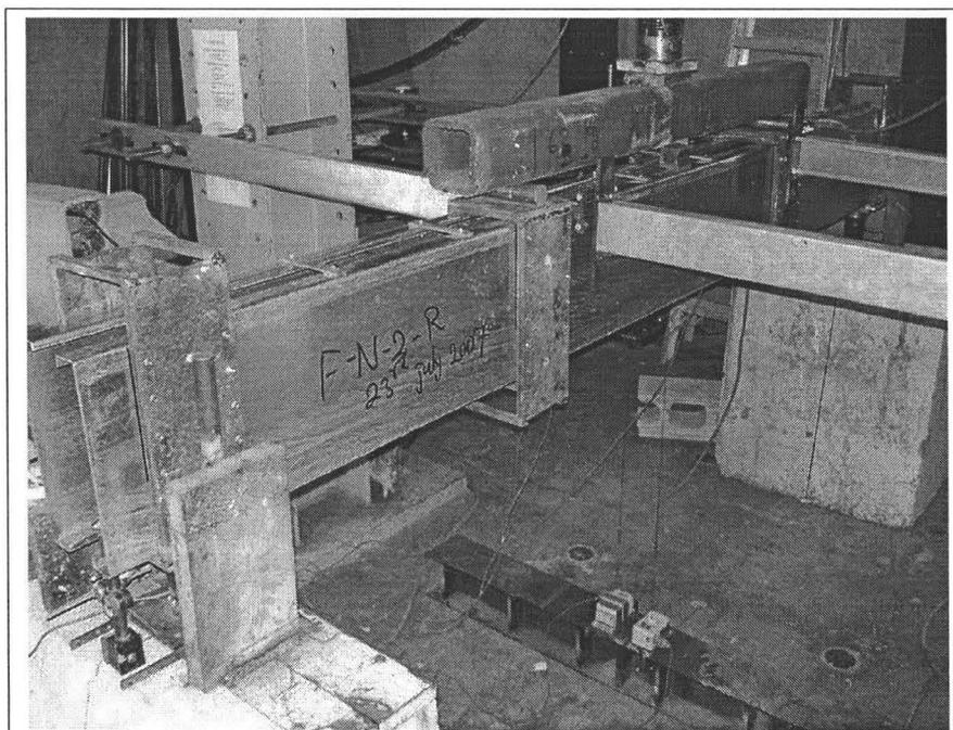
Figure 2.11: Test setup-II picture for flexure test
