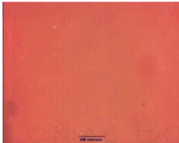
Figure 4.4 Optical transmission image of a good quality 50 nm thick YBCO film.
