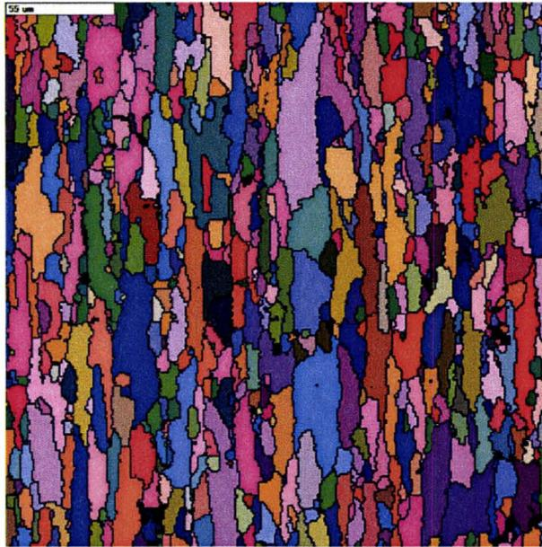
Figure 7.20: Orientation map of 6111-NC-90 quenched from 460 °C. The RD is vertical and the ND is horizontal.
