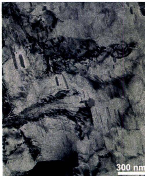
**Figure 7.6:** TEM micrograph of a 6111-NC-90 sample heated up to 400 °C at a rate of 40 °C/min.
