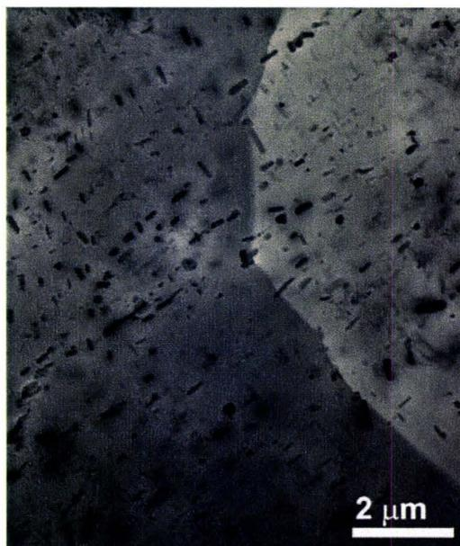
**Figure 7.7:** TEM micrograph of a 6111-NC-90 sample heated up to 460 °C at a rate of 40 °C/min.
