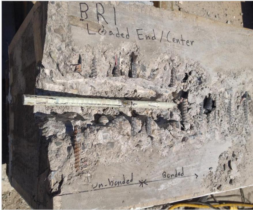
*Figure 4:12: BRI, "Test End". Marked lines on GFRP bar indicate observance of significant fibre disengagement*
