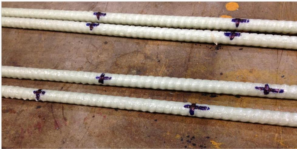
*Figure 3:5: TEME Corp. GFRP bar with ribbed surface deformations*
