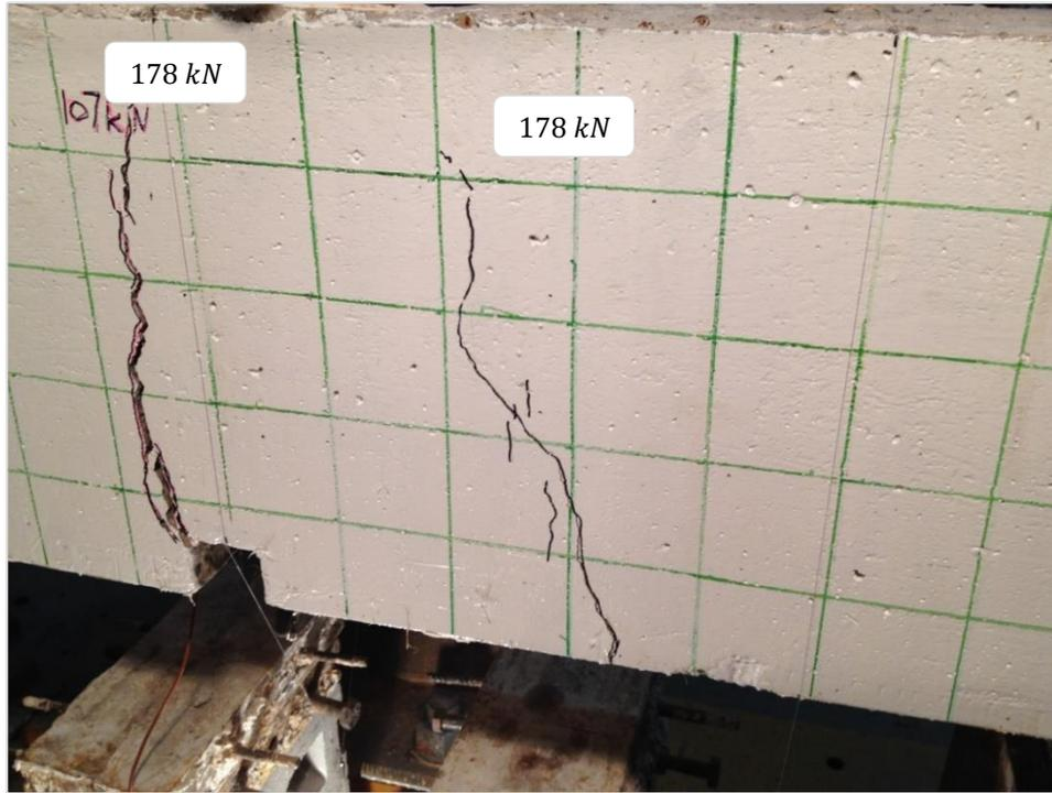
*Figure 4:21: BN1 after the second flexural crack*
