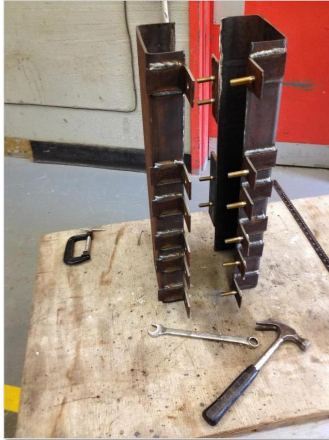
*Figure 4:37: HSS section used to provide light confinement for MP2*
