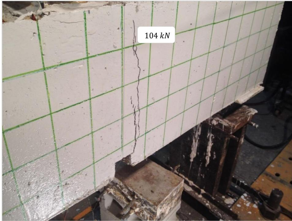
*Figure 4:24: BN2 after the first flexural crack*
