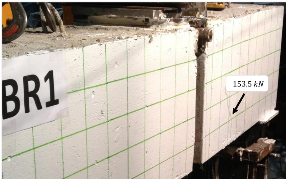
*Figure 4:4: BR1 at failure*
