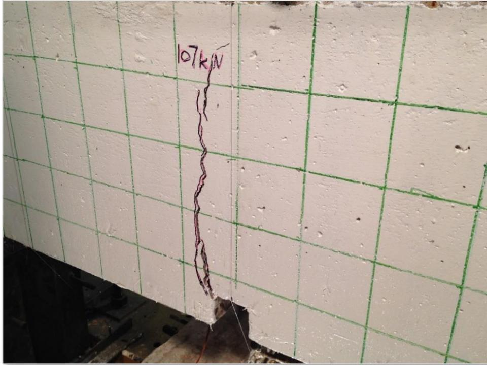
*Figure 4:20: BN1 after the first flexural crack*
