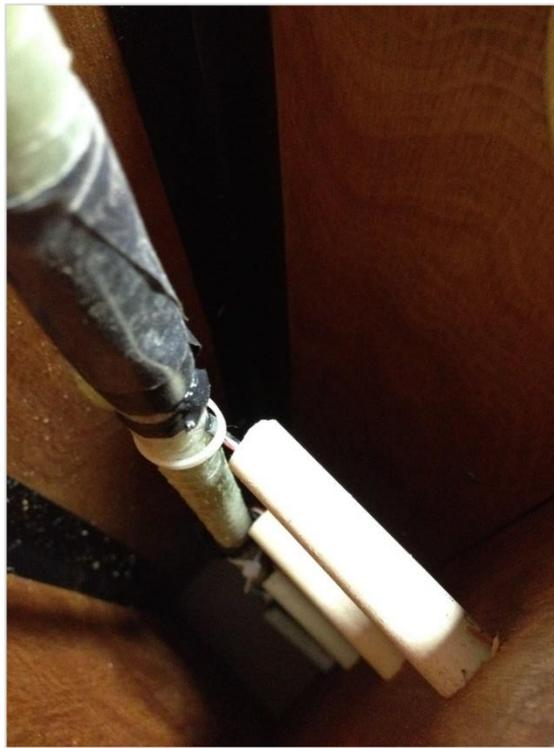
*Figure 3:23: PVC pipes used to protect the strain gauge wires in the Modified pullout specimens*
