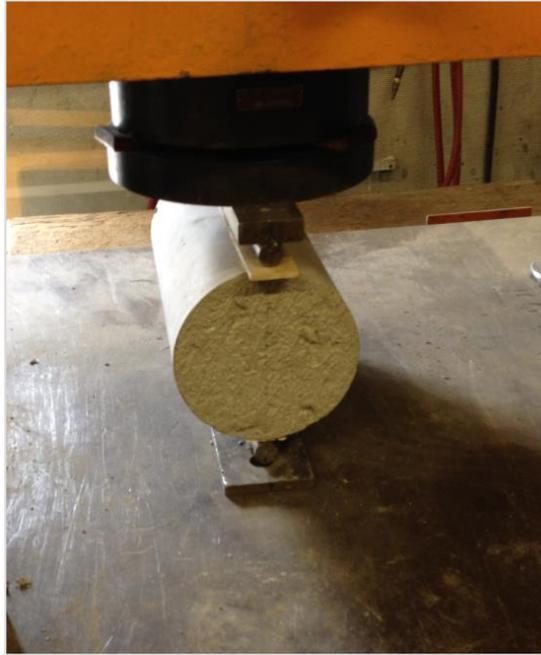
Figure 3:8: Concrete split-cylinder testing
