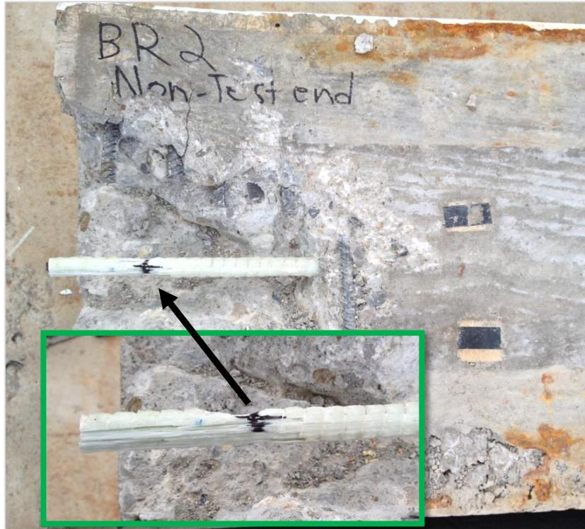
*Figure 4:18: BR2 “Non-test End”. Showing the damage and rupture experienced by the GFRP bar*
