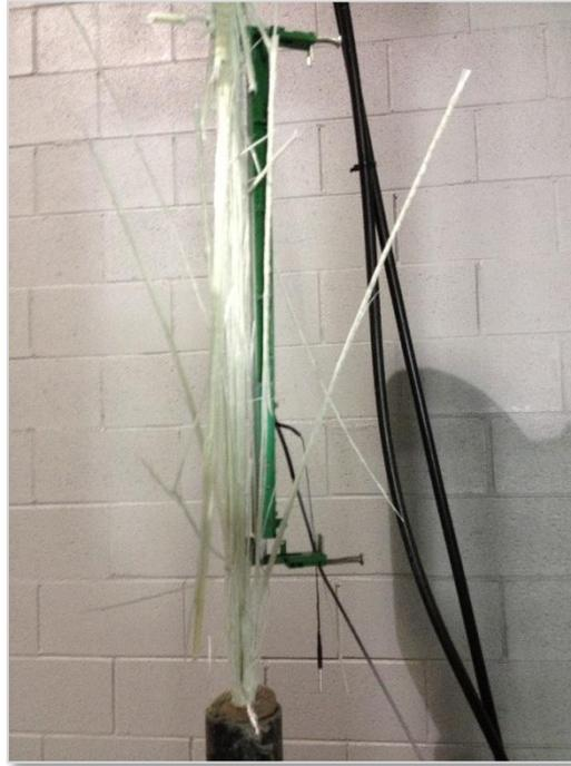
*Figure 3:4: Sudden rupture failure of GFRP bars*
