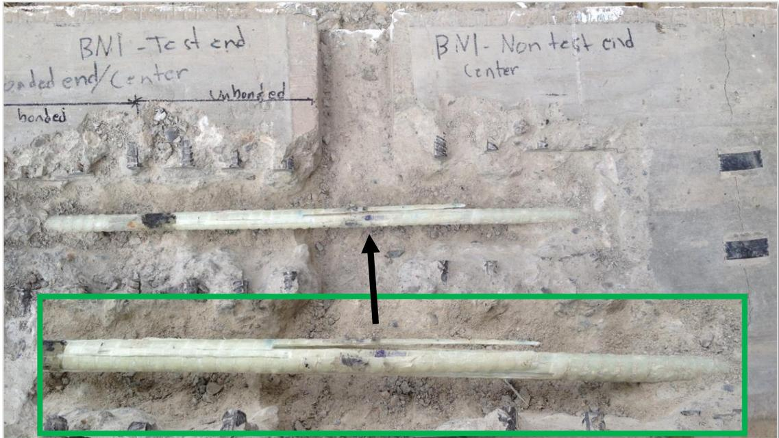
*Figure 4:32: BN1 "Test End". Showing the damage and rupture experienced by the GFRP bar*
