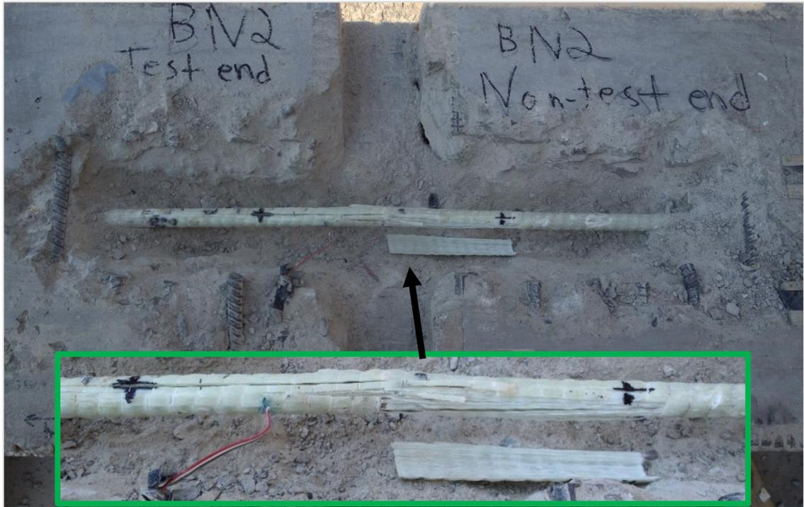
*Figure 4:34: BN2 "Test End". Showing the damage and rupture experienced by the GFRP bar*
