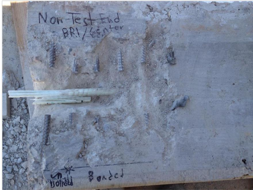
*Figure 4:14: BR1 “Non-test End”. Showing the damage and rupture experienced by the GFRP bar*
