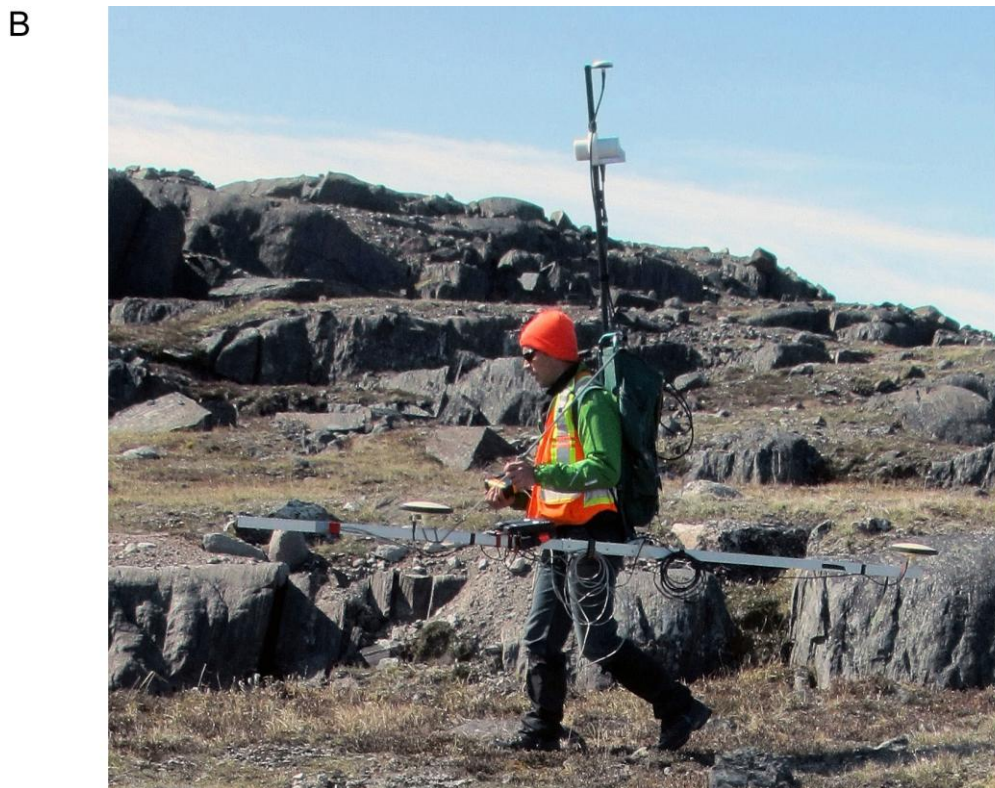
Figure 4. A) Prototype vector magnetometer system, consisting of a single fluxgate tri-axial magnetometer (Applied Physics 1540S) mounted on the end of a 2.7 m aluminum boom. A MEMS tilt sensor (OceanServer OS5000) and two D-GPS receivers (ProMark 3) also mounted on the boom recorded sensor pitch, roll and yaw (azimuth). B) Fluxgate system in use during a ground-based survey of Deposit #4 at Mary River. A second Overhauser magnetometer (GEM GSM-19) was pole-mounted on the backpack and used to record the absolute total magnetic intensity (TMI).
