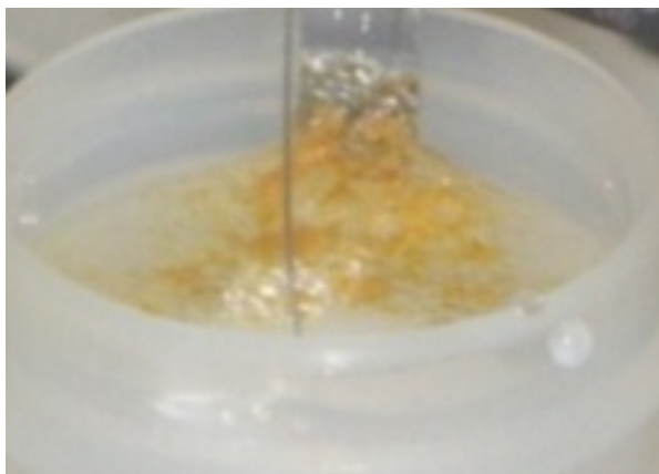
Figure 7.2. Anodized in the 8:2 (volume ratio of concentrated sulfuric acid to concentrated HF) at 20V, a layer of yellow oxide is formed on the surface and began to detach off the surface.
