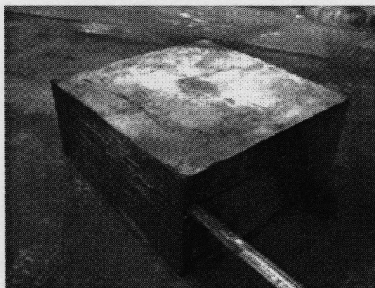
Figure 2.12. Bearing NB1 after completion of cyclic testing program; as indicated a significant delamination occurred in the bonding of one layer
