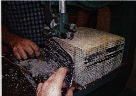
(a) Trimming the edges with an appropriate band saw
