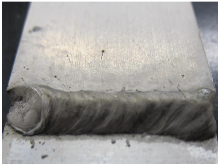
Figure E3 Close-up images of lap-joint welded configuration D (ER5356/AA7003/⊥) in the as-welded T6+PB condition post exposure to GMW-14872.
