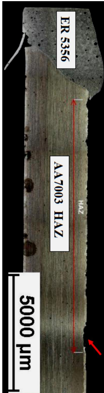
Figure 31: Large area scans of welded (a) AA7003 (configuration A1) and (b) AA7108 (configuration C1) in the as-welded T6 condition post exposure to ASTM G85-A2
