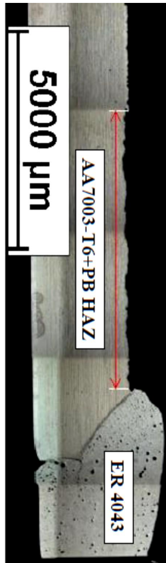
Figure D3 Large area scans of lap-joint welded configuration D (ER4043/AA7003/L) in as-welded T6+PB condition post exposure to ASTM G85-A2.
