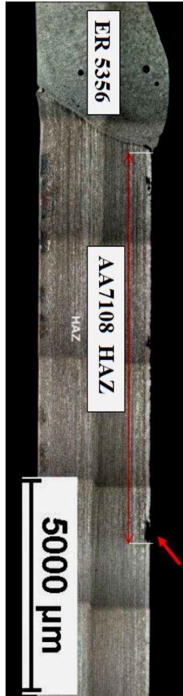
Figure 31: Large area scans of welded (a) AA7003 (configuration A1) and (b) AA7108 (configuration C1) in the as-welded T6 condition post exposure to ASTM G85-A2
