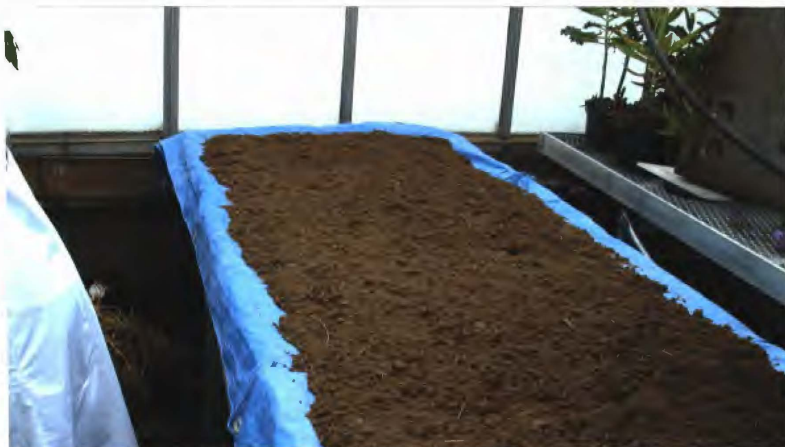
(D) Approximately 40 kg soil was spread upon a clean tarp in a greenhouse (McMaster University). Sticks, stones, and sod were removed manually from soil. Soil was covered with the tarp and allowed to air dry for 9 days.
