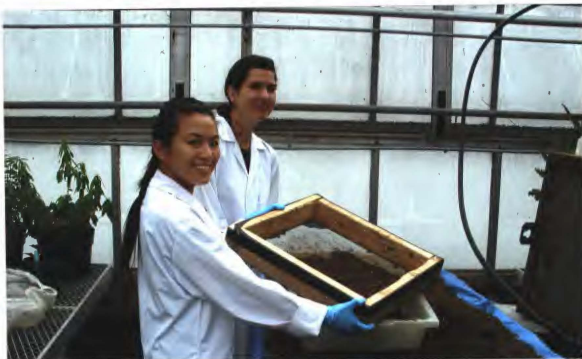
(E) Dried soil was sieved to remove particles greater than 2 mm
