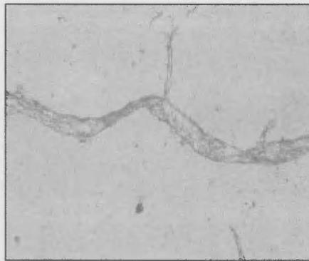
Figure 3.13 Optical microscope image of fibre after beating
