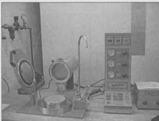
Figure 3.4 Standard 159-mm-diameter sheet machine, opened to reveal mesh on which handsheet forms. (Courtesy of Dr. R. Pelton, Chemical Engineering department, McMaster University)
