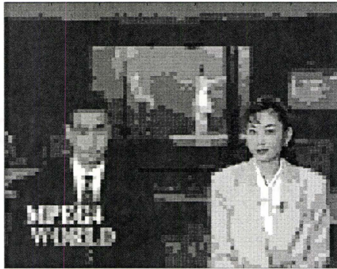
Figure 3.4: “news” image using ROI coding by multiple codebook size (unstructured VQ) with 0.3 bpp.
