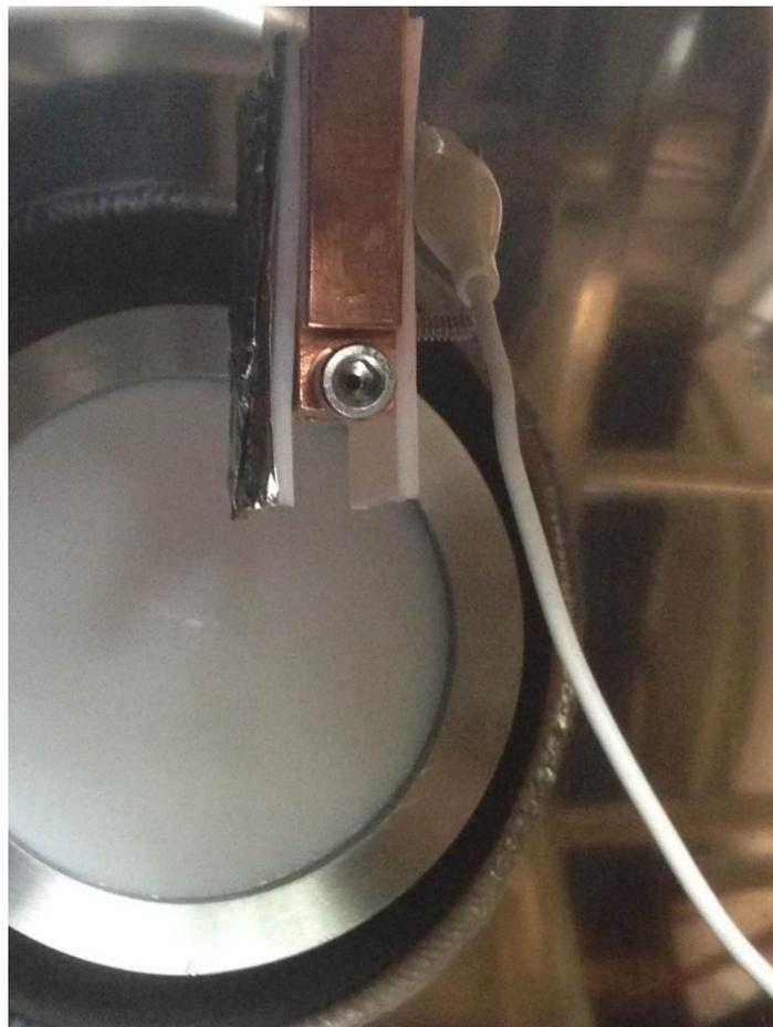
**Figure 4. 29 Aluminum film on the sample holder to collect the beam current**
