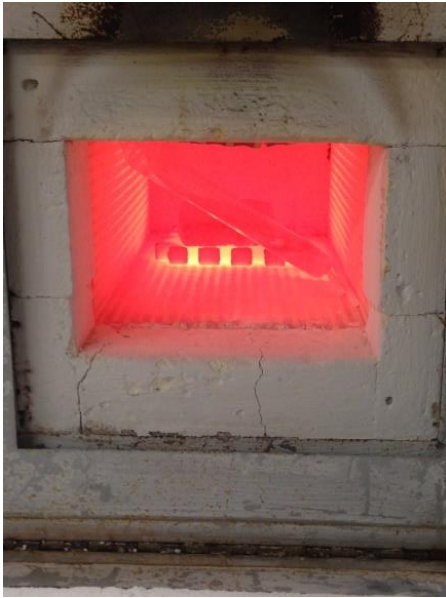
Figure 3.5: (a) Ga and Sb melt inside a box furnace
