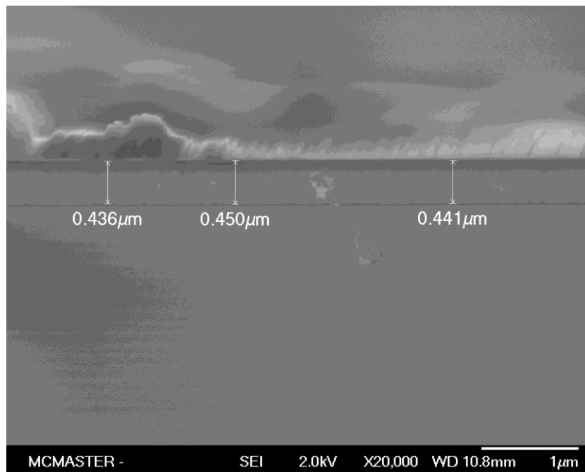
Figure 4.29: SEM Cross sectional view of Growth Attempt 18 showing film thickness
