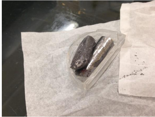
Figure 3.6: Solid GaSb placed in quartz molding crucible
