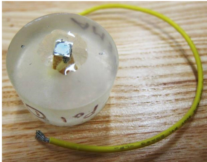
Figure 4.3: Epoxy-mounted sample with wire attached and fast-curing epoxy applied around the edges of the exposed surface.
