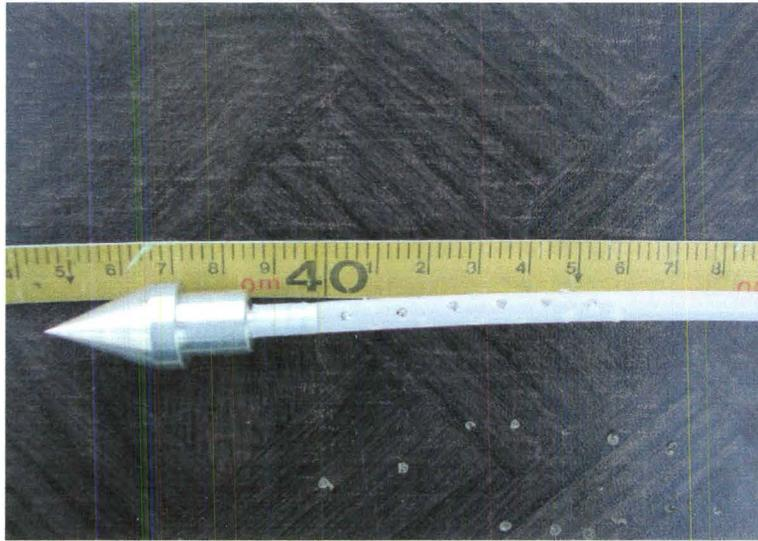
**Figure 2.7: The Sampling Point Used for Groundwater Sampling**
