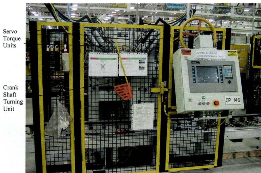
Figure 7.1B – Connecting Rods Torque Operations (OP146)
