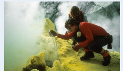
Figure 2.13: For the most accurate measurement of the type and quantity of gases being produced by a volcano, sample collection often must be made by hand. In this image, gas is being collected from Mt. Baker in Washington State, USA.
