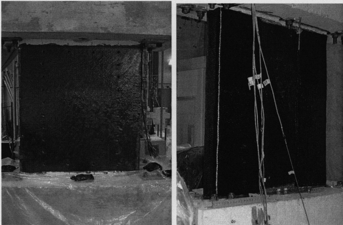
Figure 3. 15 Wall RW3 CFRP end column confinement.
