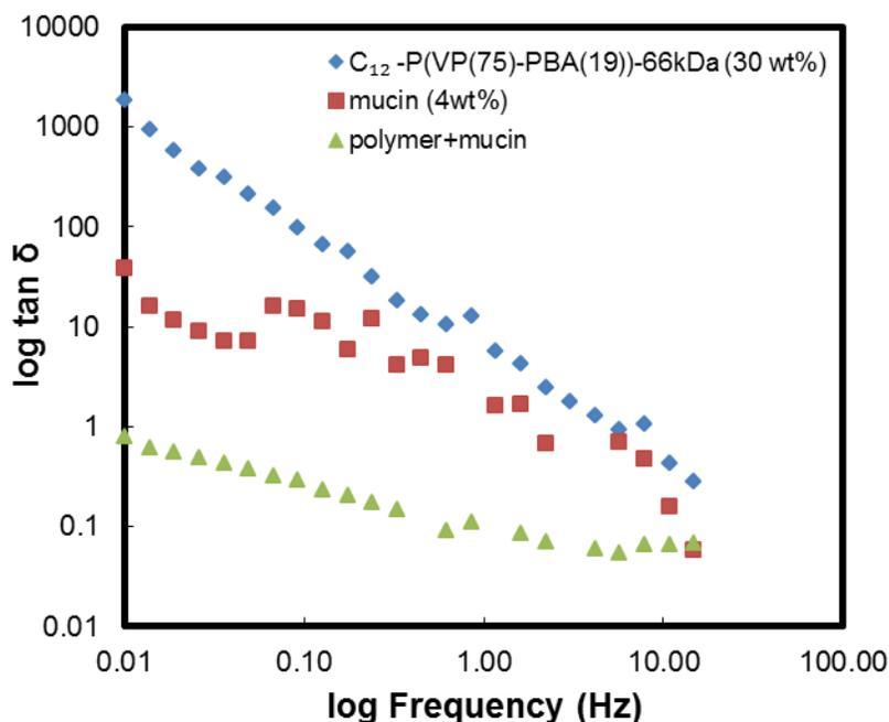
**Figure 3- 9** -  $\tan \delta$  versus frequency profile for high-PBA content  $C_{12}$ -P(VP(75)-PBA(19))-66kDa) dual  $C_x$ -PBA grafted polymer (30 wt%) in the absence and presence of mucin (4 wt%)
