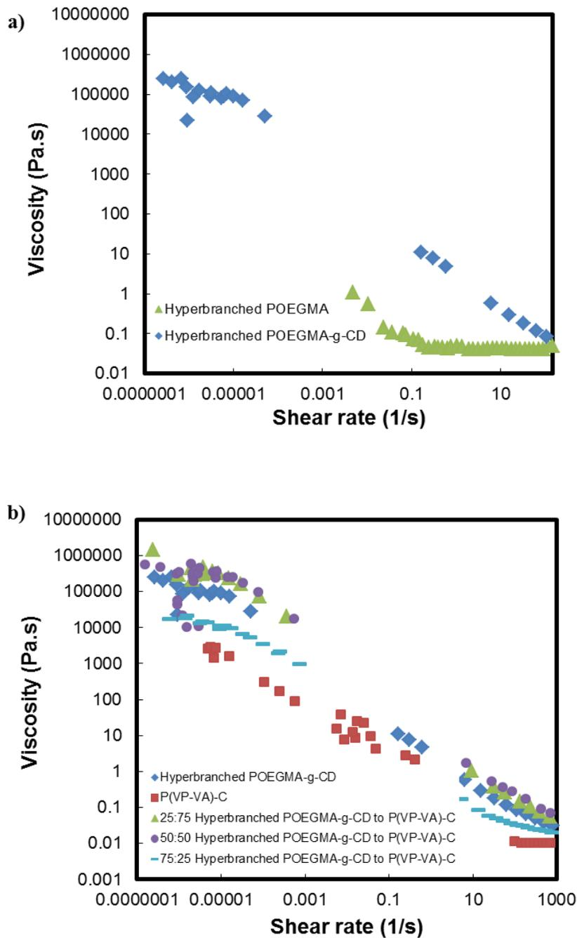
**Figure 2- 12-**Rheology of CD-grafted hyperbranched polymer (10.4 mole% EGDMA, 3.7 mole% DDT): (a) comparison of viscosity profile of hyperbranched polymer before and after CD grafting; (b) rheology of mixtures of linear hydrophobically grafted poly(N-vinylpyrrolidone) linear polymers (55 kDa molecular weight, 1.7 mol % C<sub>x</sub> hydrophobes) mixed with CD-grafted hyperbranched polymer
