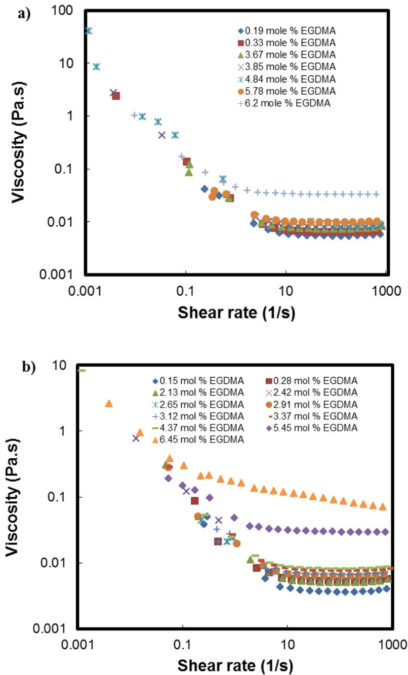
**Figure 2- 8-**Viscosity versus shear rate as a function of increase in EGDMA content for hyperbranched polymers prepared with a) 1.2 mole % DDT and b) 1.4 mole % DDT
