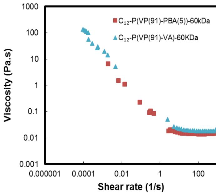
Figure 3- 4-Viscosity versus shear rate of  $C_{12}$ -P (VP-VA)-60kDa before and after PBA conjugation
