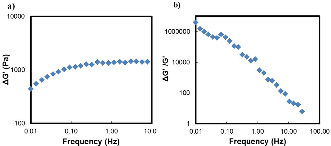
**Figure 3- 10** – Representative example of a) excess storage modulus and (b) relative synergism parameter or  $C_{12}$ -P(VP(75)-PBA(19))-66kDa measured as a function of frequency for dual  $C_x$ -PBA grafted polymers
