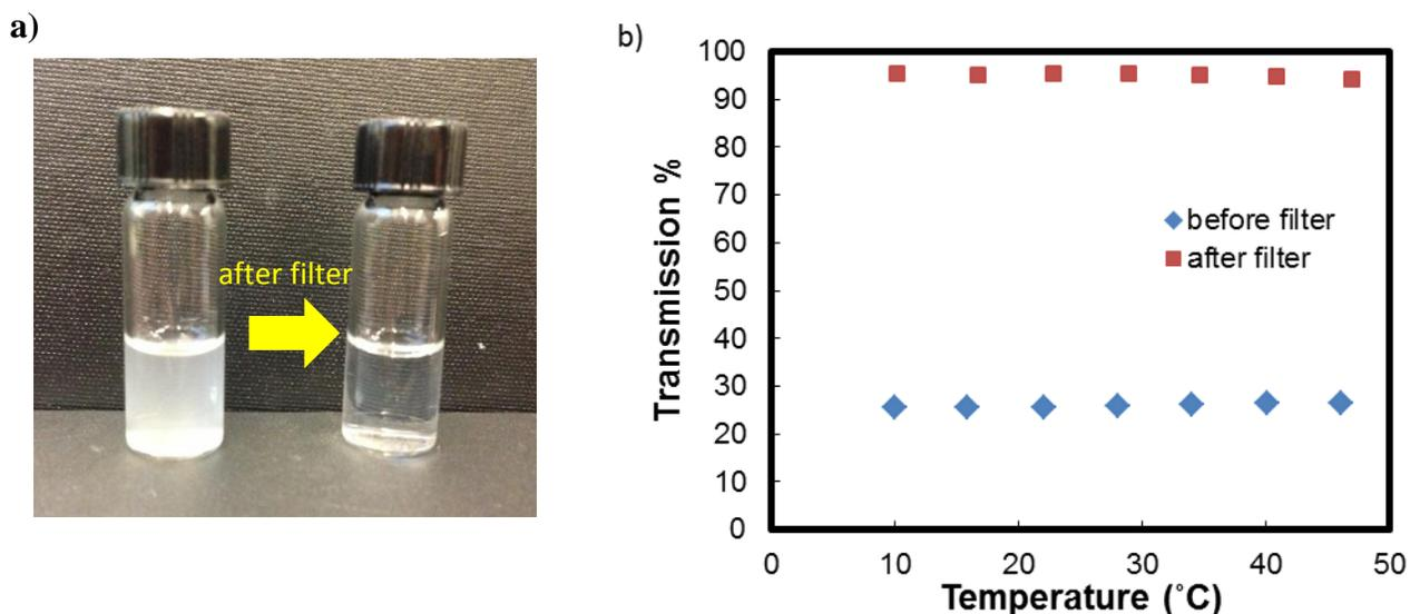
**Figure 2- 6-**(a) Visual appearance and (b) UV/vis transmittance value at 500 nm wavelength for a 15wt% solution of hyperbranched polymer with 1.45 mol % DDT and 6.2 mol % EGDMA
