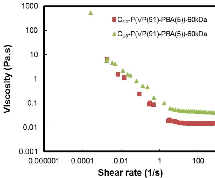
Figure 3- 5-Viscosity versus shear rate of dual  $C_x$ -PBA grafted P(VP(91)-PBA)-60kDa polymer functionalized with different hydrophobe chain lengths
