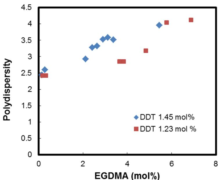
**Figure 2- 4**-Effect of increasing the EGDMA (cross-linker) concentration on hyperbranched polymer polydispersity at two different DDT (chain transfer agent) concentrations
