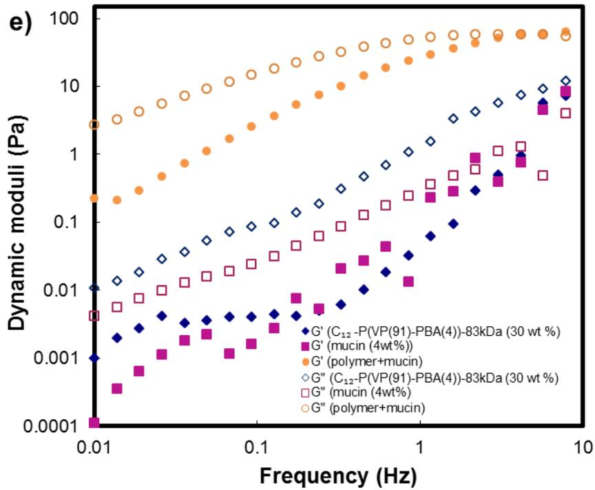
**Figure C 1-** Dynamic oscillation responses of dual  $C_x$ -PBA grafted polymers for a) P(VP(90)-PBA(5))-60kDa (30wt%), b)  $C_{12}$ -P(VP(91)-PBA(5))-60kDa (30 wt %), c)  $C_{18}$ -P(VP(91)-PBA(5))-60kDa (30 wt %), d)  $C_{12}$ -P(VP(84)-PBA(13))-65kDa (30 wt %), e)  $C_{12}$ -P(VP(91)-PBA(4))-83kDa (30 wt %),
