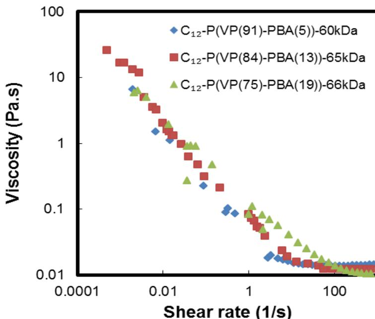
**Figure 3-7**-Viscosity versus shear rate of dual C<sub>x</sub>-PBA grafted C12-P (VP-PBA) polymers with different PBA contents
