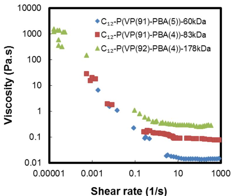
**Figure 3- 6-**Viscosity versus shear rate of dual  $C_x$ -PBA grafted  $C_{12}$ -P(VP-PBA) polymers with different molecular weights
