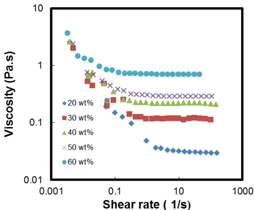
**Figure 2- 10-**Viscosity versus shear rate for hyperbranched polymer 20 (6.45 mole% EGDMA,1.45 mole% DDT) as a function of polymer concentration
