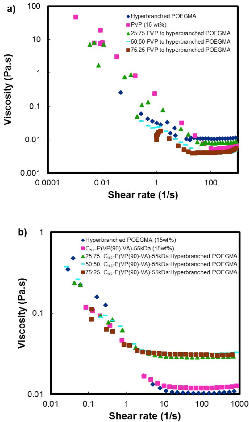
**Figure 2- 11-** Rheology of hyperbranched polymer (10.4 mole% EGDMA, 3.7 mole% DDT) mixed with (a) PVP (b) linear hydrophobically grafted PVP linear polymers (55 kDa molecular weight, 1.7 mol % C<sub>12</sub> hydrophobes) mixed with CD-grafted hyperbranched polymer
