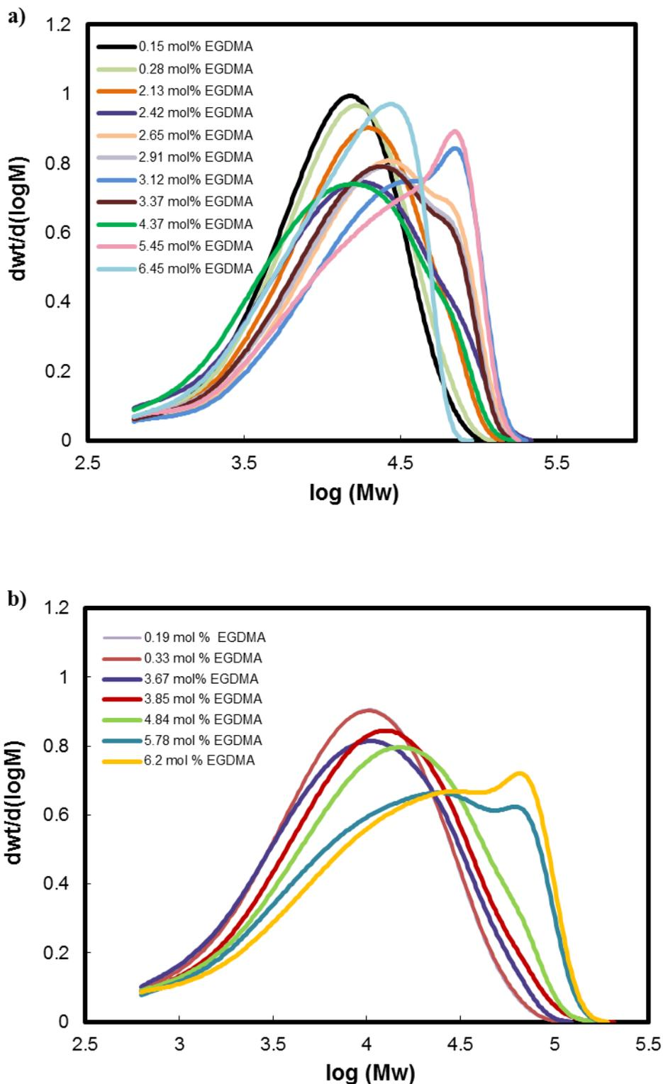
**Figure 2- 5-**Molar mass distribution curves of hyperbranched polymers (from GPC refractive index detection) for polymers prepared with different concentrations of EGDMA and a)1.23 mole % of DDT and b)1.45 mole % of DDT
