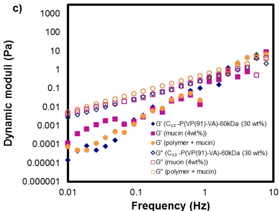
**Figure 3- 8**-Examples of dynamic oscillation responses of dual  $C_x$ -PBA grafted polymers for a) a polymer with low PBA content ( $C_{12}$ -P(VP(90)-PBA(4))-178kDa) and b) a polymer with high PBA content ( $C_{12}$ -P(VP(75)-PBA(19))-66kDa) and c) a polymer with no PBA conjugation ( $C_{12}$ -P(VP(75)-VA)-66kDa)
