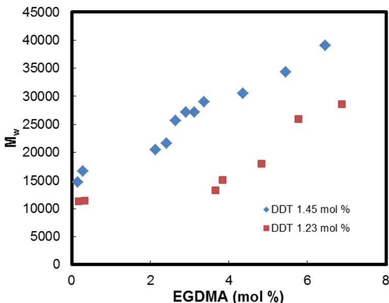
**Figure 2- 3**-Effect of EGDMA (cross-linker) mole percentage on hyperbranched polymer  $M_w$
