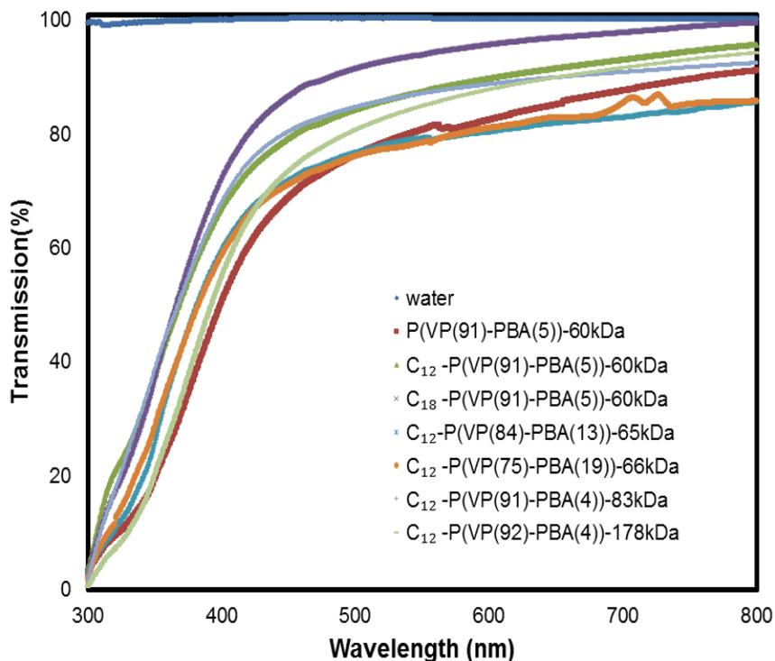
**Figure 3- 2-**Transmittance of polymers as a function of wavelength (15 wt % solutions)
