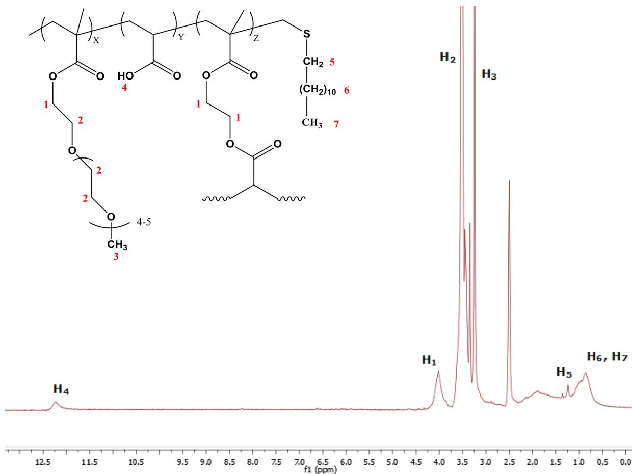
**Figure 2-**  $^1\text{H}$  NMR spectrum of hyperbranched POEGMA-co-AA synthesized with EGDMA as the cross-linker and DDT as the chain transfer agent
