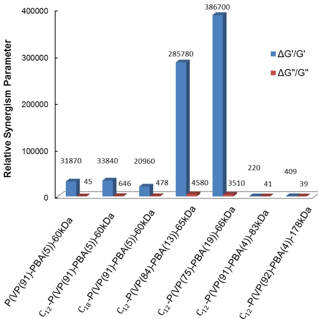
**Figure 3- 11** – Rheological synergism of polymer-mucin interactions: (a) excess modulus ( $\Delta G'$ , blue series, or  $\Delta G''$ , red series); (b) relative synergism parameter ( $\Delta G'/G'$ , blue series, or  $\Delta G''/G''$ , red series)
