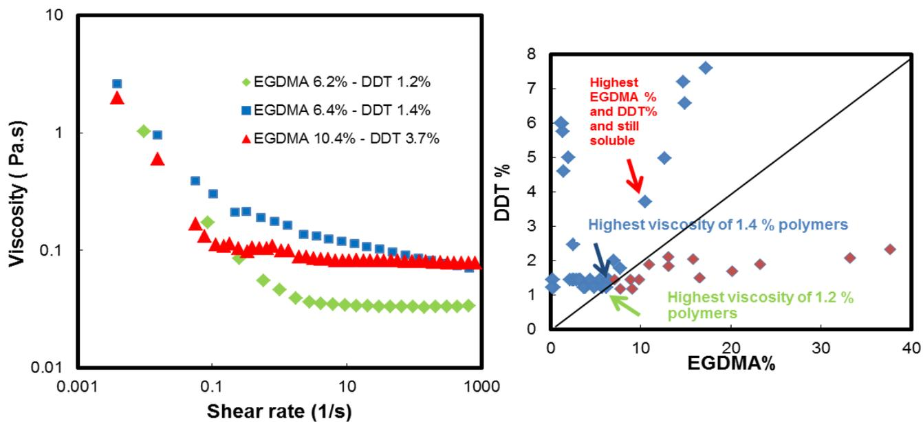
**Figure 2- 9**-Rheological comparison of hyperbranched polymers prepared with the highest EGDMA content and 1.45 mole% and 1.23 mole% DDT (from Figure 2-5) with the hyperbranched polymer prepared with the highest EGDMA and DDT contents resulting in a soluble hyperbranched polymer (EGDMA 10.4%-DDT 3.7%); Inset: polymer composition map showing location of the three polymers considered in the sample space
