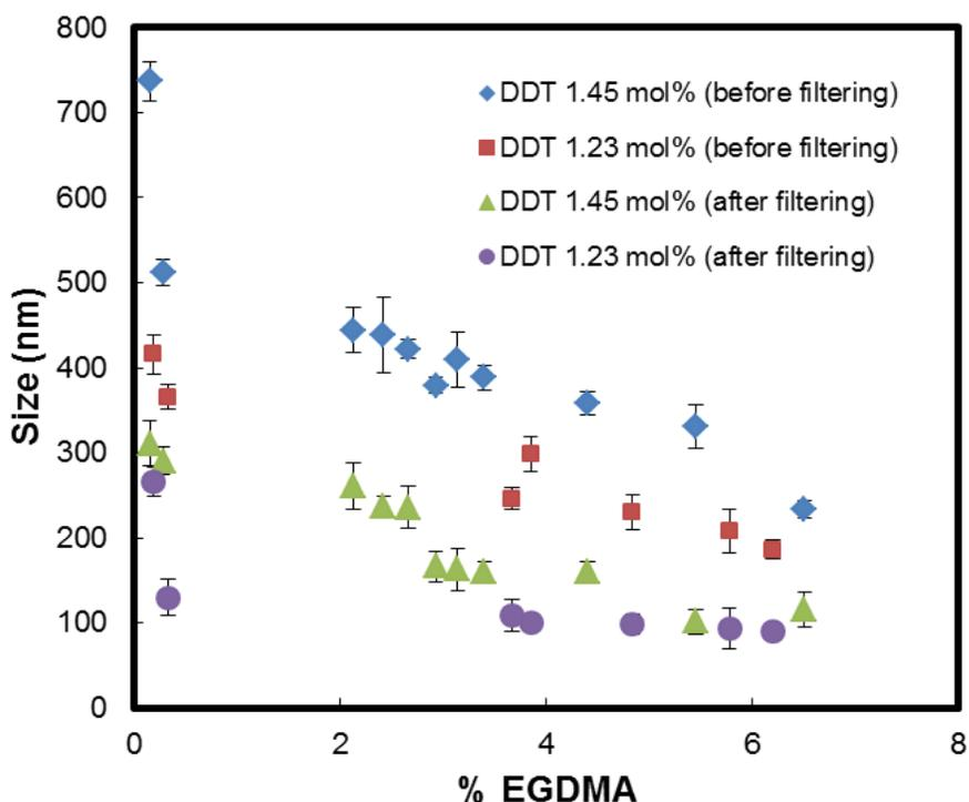
**Figure 2- 7**-Hydrodynamic diameter of hyperbranched polymers prepared with varying EGDMA (cross-linker) contents at fixed DDT (chain transfer agent) concentrations before and after sample filtration
