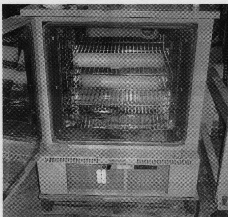
Figure B.2 Pre-heating of billets in external oven.
