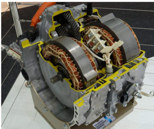
(a) Toyota Hybrid System – Input split
