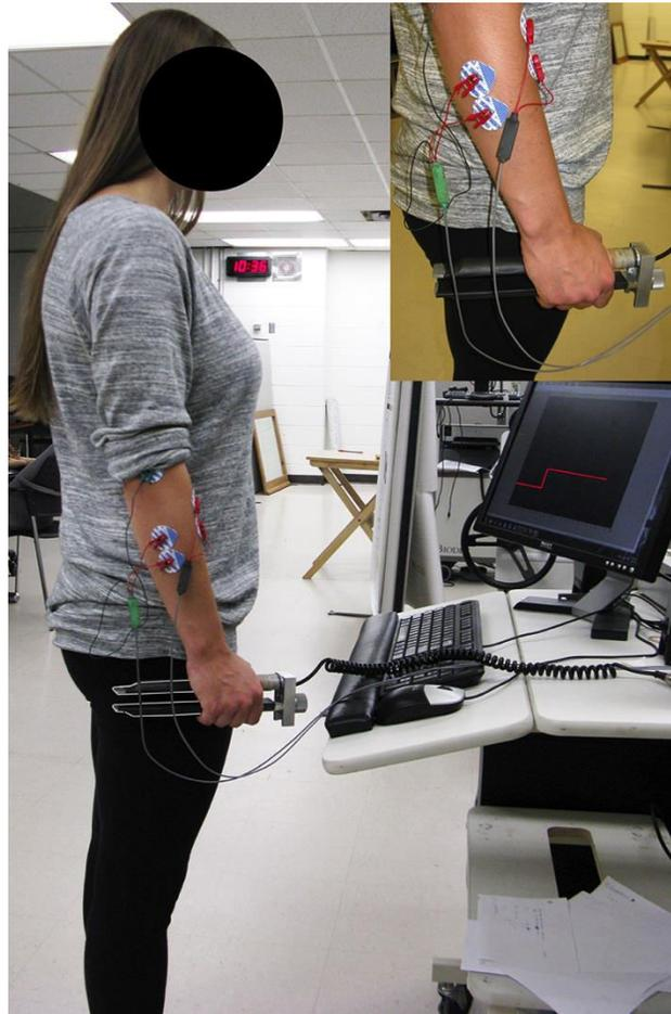
**Figure 3.1.** Participants held the handgrip dynamometer at their side, with the wrist in a neutral posture. Participants were instructed to trace a template on a computer monitor by squeezing the dynamometer to match a red line with a grey template line. During the trial, the participants were instructed to keep the hand by the side, the arm close to the body, and the webbing of the thumb positioned on the dynamometer at the same place throughout the trial.
