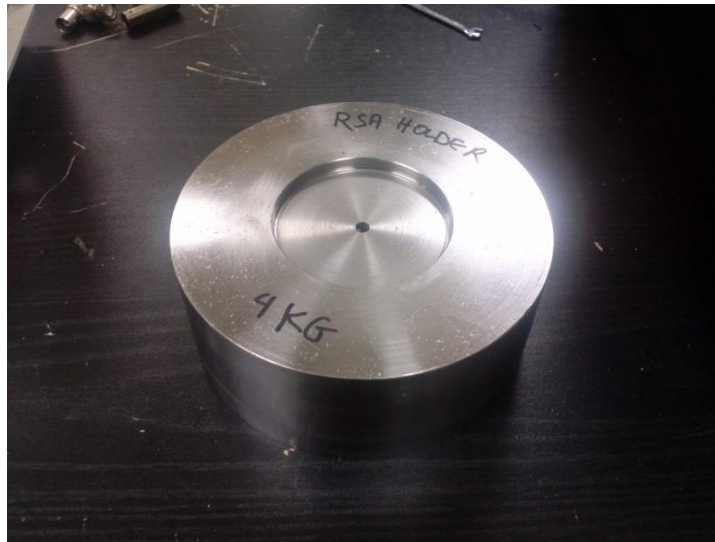
Figure 3.3 Steel Workpiece Holder for RSA-6061 Workpiece, 4kg Mass
