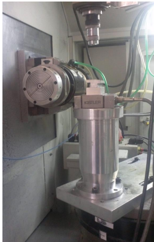
Figure 4.1 Tool-Holding Fixture, Before Modifications
