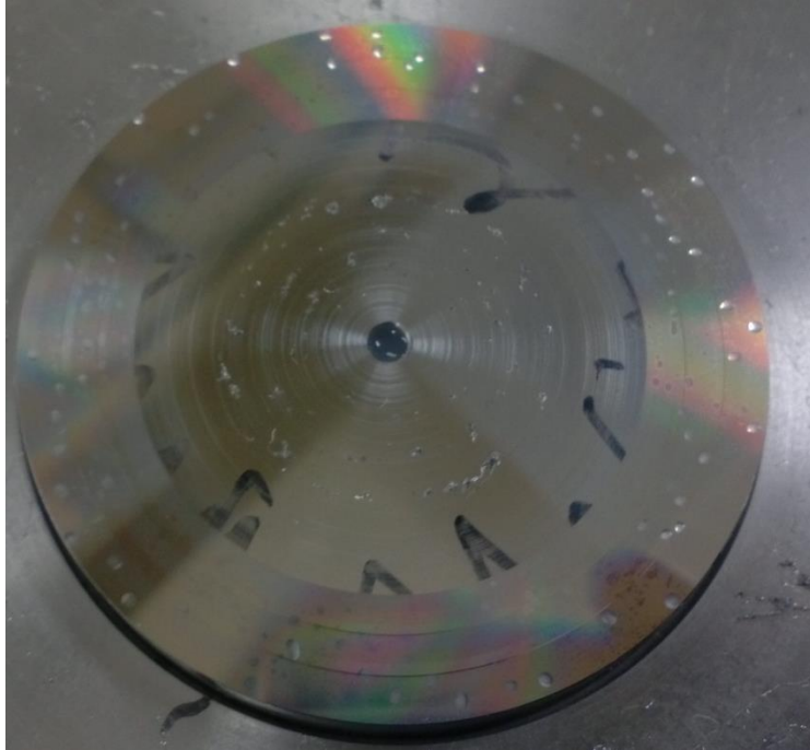
Figure 5.25 Example of Diffraction Grated Surface on Workpiece
