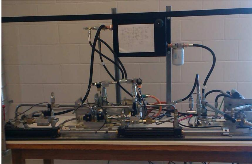
Figure 5.2: Experimental setup of the electro-hydrostatic actuator (EHA): The piston on the right is referred to as piston *A* (3) and the piston connected to it on the left is referred to as piston *B* (4). An optical linear encoder (12) attached to piston *A* is used to provide position measurements (which are differentiated to obtain velocity measurements). The gear pump (10) and electric motor (13) are located in the rear (middle) of the table.
