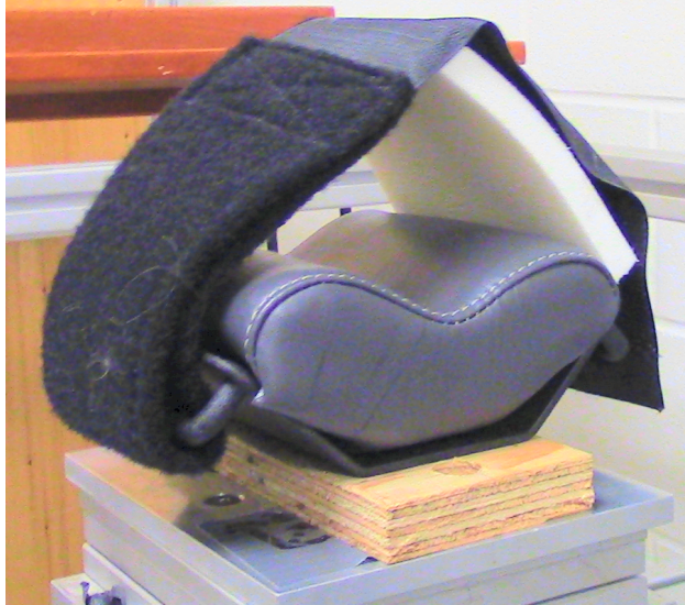
Figure 3.3: The custom padded arm strap apparatus is seen here. The participant rested their humerus inside the cuff, and then the padded arm strap was secured on the humerus just proximal to the elbow.
