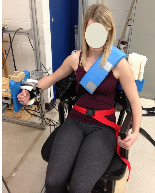
Figure 5.1: The umbilicus 60° hand location is shown. This and the eye 45° hand locations, both elicited this abducted and extended arm posture. This creates a large moment arm from the hand to the shoulder, which emphasizes the importance of the humeral rotation strengths to maintain the arm posture during certain exertions.
