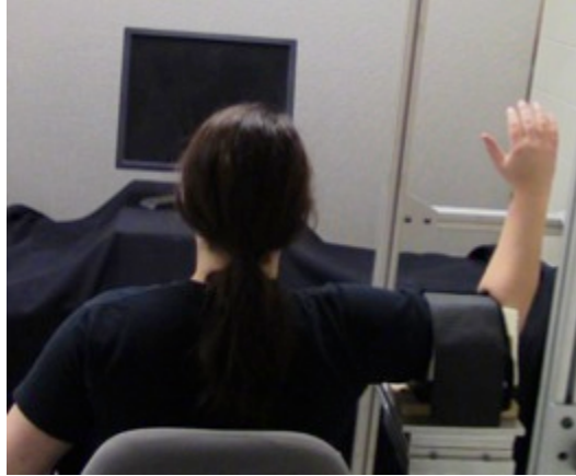
Figure 2.18: The arm posture used by Hodder & Potvin (2014) to test the WAA and IAA. Participants were seated in a chair with their arm in 90° of abduction with the elbow flexed to 90° such that the forearm was in a vertical position. All of the required exertions were completed while in this same posture. The arm brace that was used was full padded and its position could be adjusted to accommodate a wide range of participant anthropometrics.
