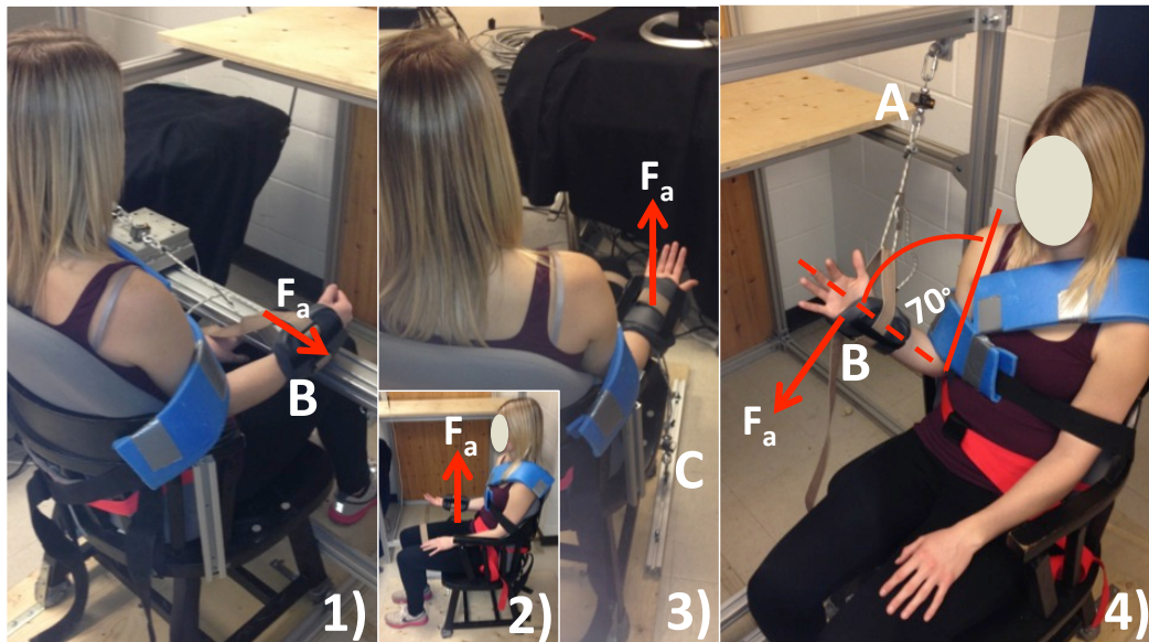
Figure 3.6: This diagram shows several views of the lateral humeral rotation (1), elbow flexion (2 & 3), and elbow extension (4) JAS tests, as seen in Figure 2.1, pictures 1, 2 & 8, respectively. All of these strengths were tested while the humerus was in a neutral position with the elbow in 90° of flexion, except for elbow extension, which starts with the elbow in 70° of flexion. The red arrows indicate the direction of the applied force ( F_a ). A) the linear force transducer mounted to the inferior surface of the horizontal 80/20 rail, B) the padded wrist cuff, C) the linear force transducer attached directly below the wrist to the piece of slotted rail that is fixed to the baseboard of the chair.
