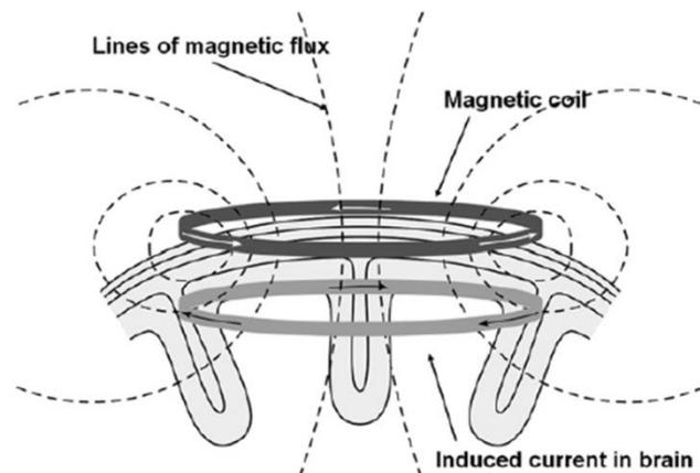
**Figure 1. TMS Magnetic Induction**
