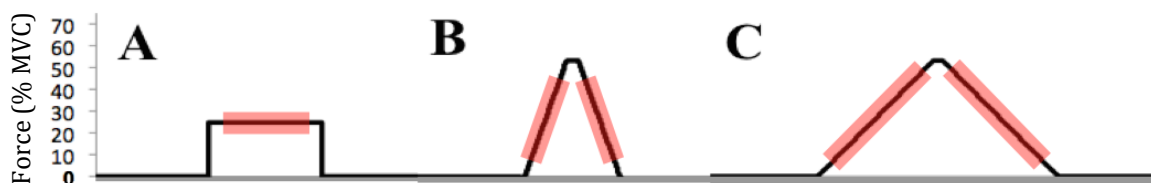
Figure 3.5. Schematic of one exertion from each submaximal trial: (A) Isotonic, (B) 2 second ramp, (C) 5-second ramp. Highlighted areas signify the middle 80% of each phase, where error and correlation measures were performed.
