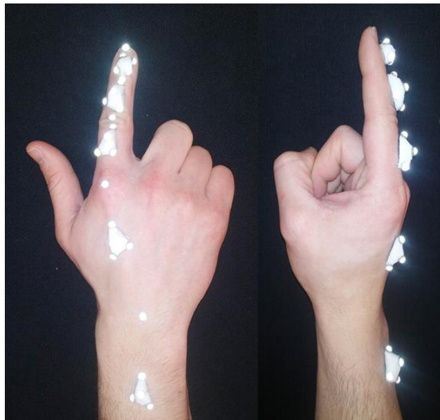
Figure 3.5 Five clusters of reflective markers placed on the dorsal surface of each segment: distal phalanx, middle phalanx, proximal phalanx, metacarpal and forearm.
